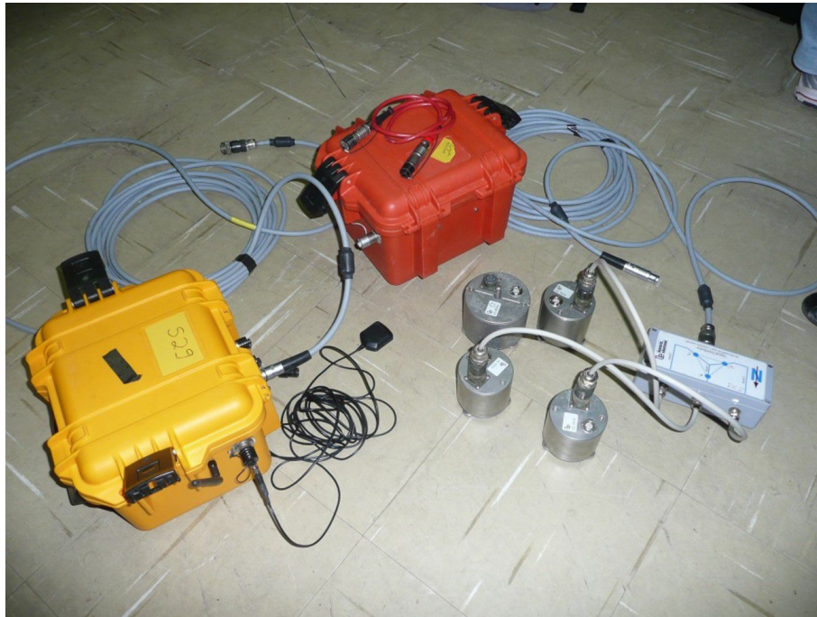
Figure 1.3: Typical components of a local short-period seismic array: 4 seismometers, data logger (in yellow box), power supply (in red box), geophone cables.
