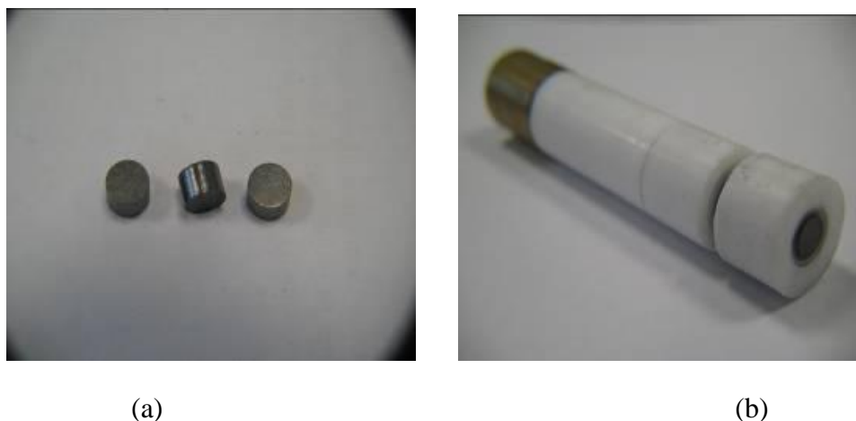
Fig.4.1: (a) Carbon composite sample electrodes - (b) mounted on a RDE holder.
