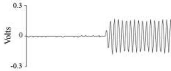
Figure S3. Start of a sound pulse used in moth electrophysiology experiments, recorded using a second transducer. The sine wave recorded was as expected, and so no extra frequencies were being created. This was the same for the range of frequencies tested. The above example is a 200 kHz sound pulse.
