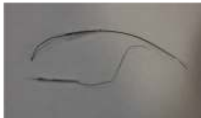
Figure A2.1 First type of electrodes produced for use in the electrophysiology experiments, the tungsten wire is placed in a glass capillary.
