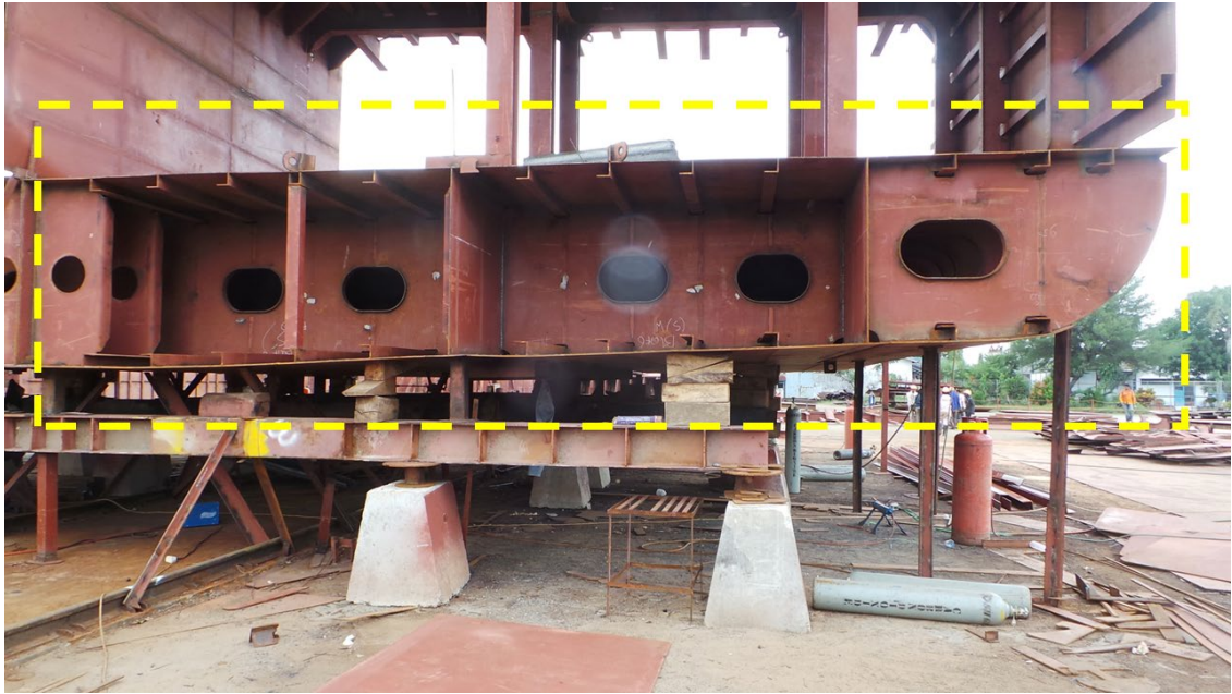
Figure 6-1 Representative environment of a ship's double-bottom confined space, illustrating the severe kinematic and accessibility constraints faced during assembly. The narrow manhole access (as seen in the lower compartment) dictates the maximum physical dimensions for robotic deployment, while the 1.2 m vertical clearance presents significant safety and ergonomic hazards for manual labour, necessitating a transition to automated welding solutions. (Note: This photograph was taken during a ship production supervision project conducted by the authors and the team from Institut Teknologi Sepuluh Nopember).
