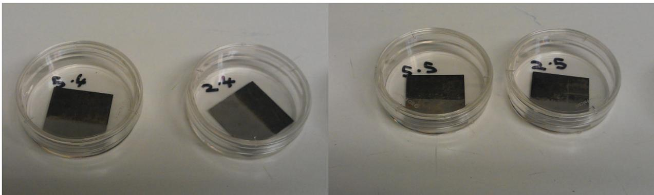
**Figure 3.2.:** NaCl-P surfaces prior to sterilisation in alcohol. Note the poor quality of coating, particularly on surface 2.5, as well as signs of steel oxidation on surface 5.5. (Used in experiments shown in Fig. 3.5:- 5.4: 5 day, no NaSa. 2.4: 2 day, no NaSa. 5.5: 5 day, plus NaSa. 2.5: 2 day, plus NaSa)
