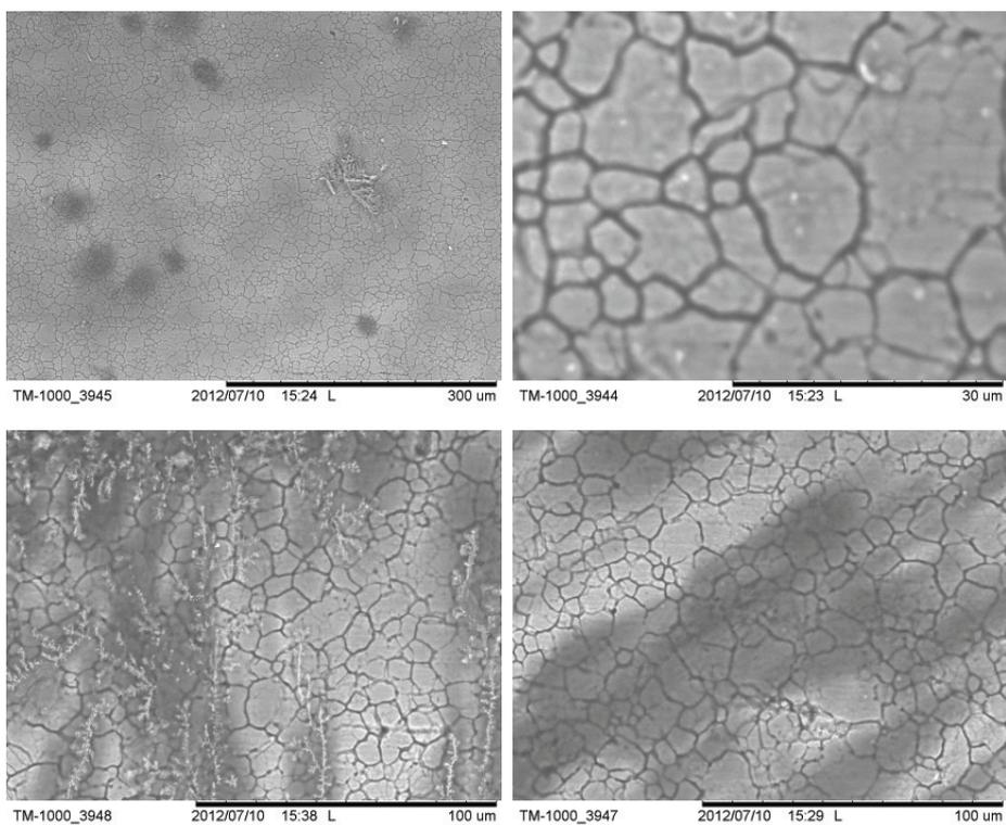
**Figure A.4.:** As discussed in sec. 3.4 Areas of poor growth on NaSa-C (top) contrasted with areas of strong growth on the same polymer (bottom)
