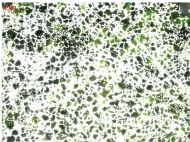
**Figure 3.6.:** Scratches on the metal surface in the crossover region on sample 2.4 (*NaCl-P for the two day time point with no NaSa added*)
