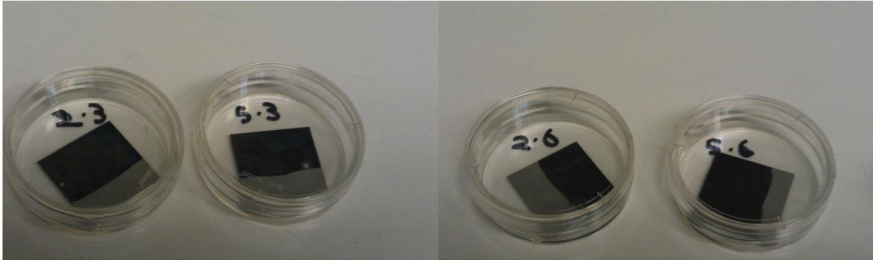
**Figure 3.1.:** Surfaces synthesised using NaSa dopant ions. (Used in experiments shown in Fig. 3.7 and Fig. 3.8:- 2.3: 2 day, NaSa-P. 5.3: 5 day, NaSa-P. 2.6: 2 day, NaSa-C. 5.6: 5 day, NaSa-C)
