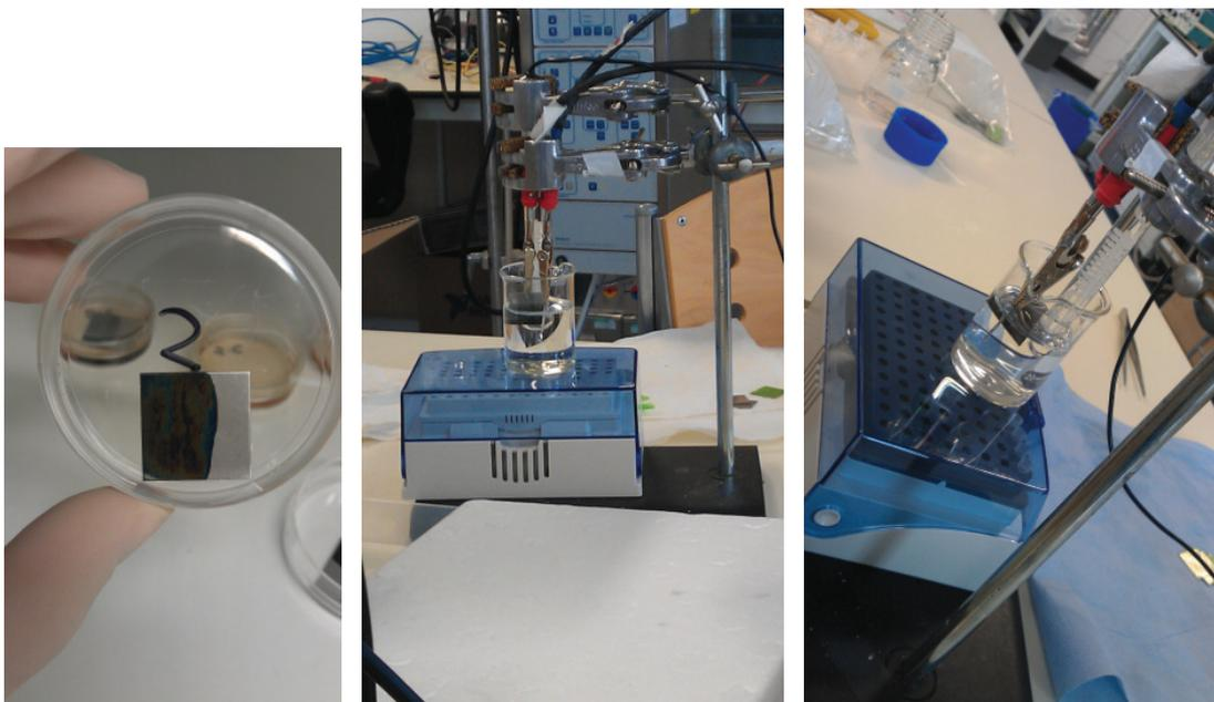
**Figure 2.1.:** Left: An example of a coated stainless steel foil, as used experimentally.
