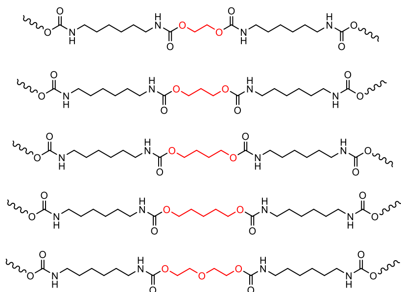
Figure 5-21. The increase of the size of hard blocks with the increase of the length of CE.
