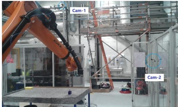
**Figure 3.12:** Location of two camera installations within the experimental environment. Each camera provides an orthogonal view relative to the other to cover for occlusions caused by the robot invading the view of the cameras.
