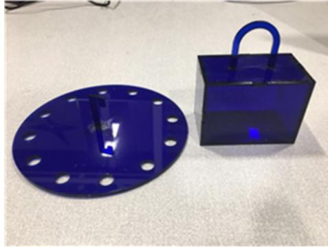
**Figure 3.10:** The hook end effector and box object used for the pick and place task. Both parts were produced through laser-cutting.
