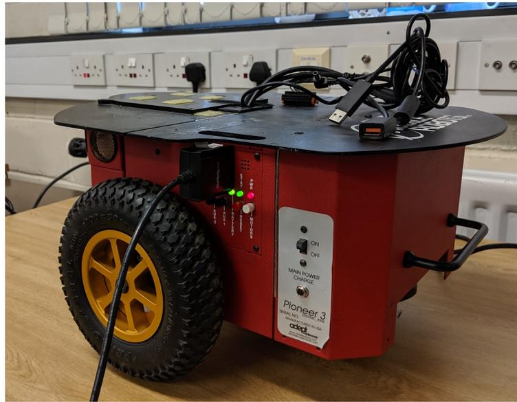
**Figure 5.11:** The Pioneer 3-DX differential drive mobile robot
