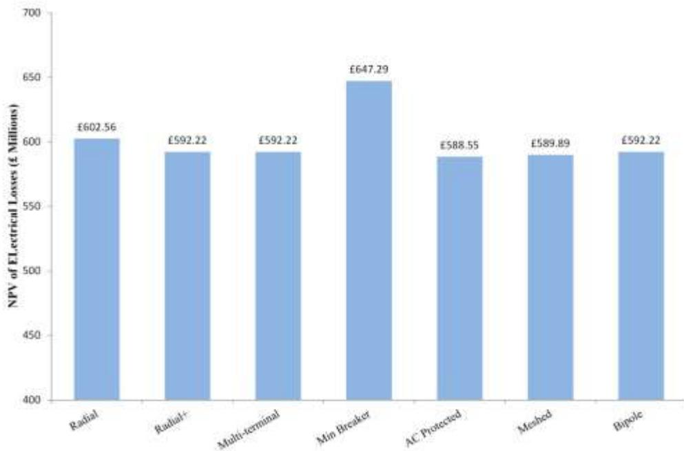
Figure 4.18 - NPV of electrical losses for Dogger Bank case studies
