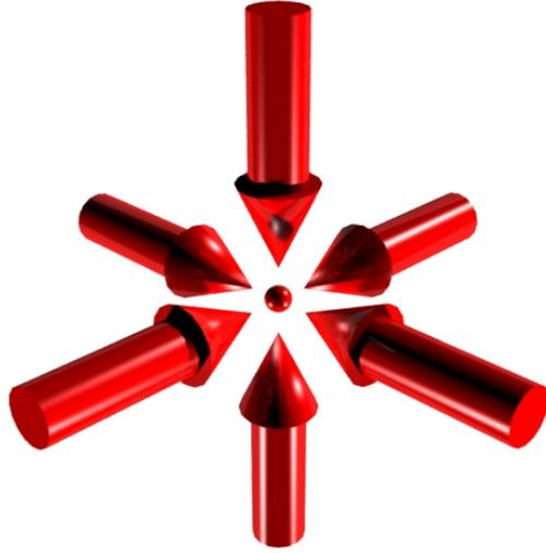
Figure 3.2: Three dimensional optical molasses. The setup of orthogonally orientated 3 pairs of red-detuned laser beams provide a syrup-like photon environment that interacts with atoms present in the cross section of all laser beams.
