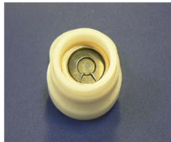
A view from overhead showing the valve placed inside the bottom half of the valve holder
