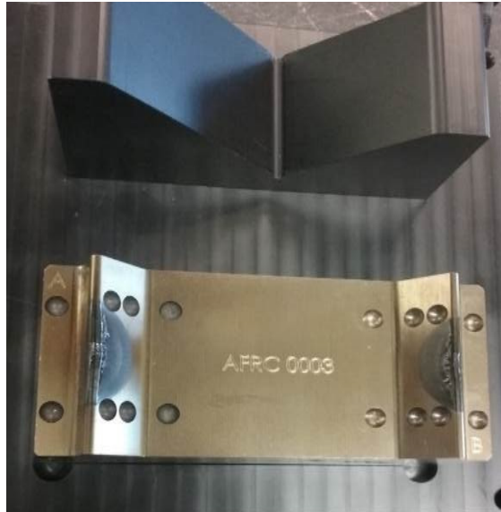
Figure 3-11: Fixture for Scanning an insert on Infocus Optical Microscope
