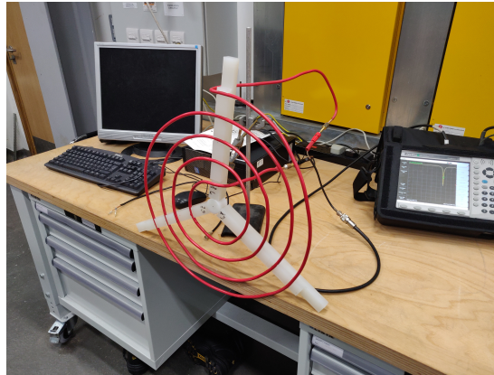
Figure 3.14: Bench testing of the helicon antenna .
