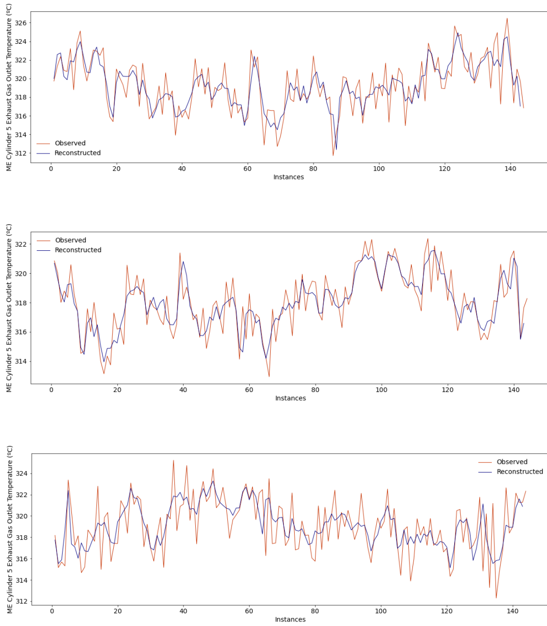
Fig. D.6.10. Example of reconstructed sequences with collective anomalies.
