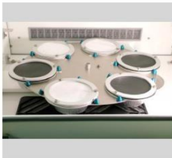
Figure 5.34 Image of sample loading method in test chamber (image taken from www.gintronic-instruments.com ).
