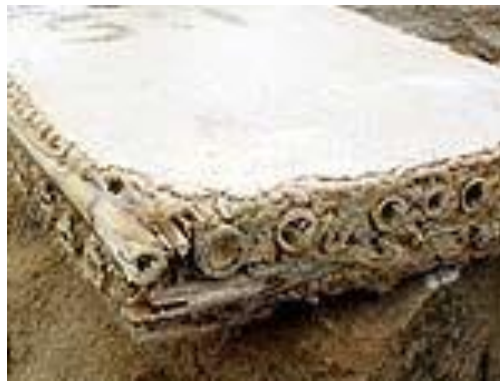
Figure 5.32 Image of the clay, reed and hessian composition of Clay board ( www.womersleys.co.uk/acatalog/Building_Products_2_6.html ).
