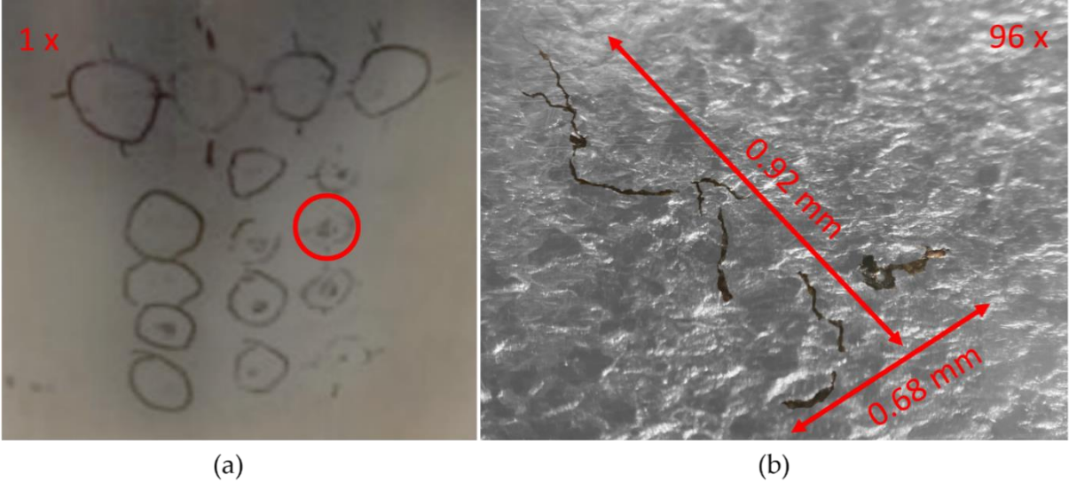
Figure 72. Photo of crack matrix and micrograph (a) Photo of crack matrix with the defect of interest highlighted in a red circle (b) Micrograph of the defect of interest at 96x zoom with desaturated background
