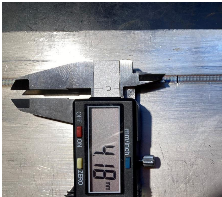
Figure 73: Illustration of EDM notched flat plate RSW sample
