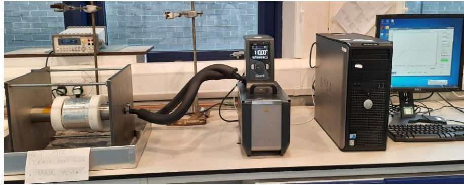
Figure 4.8 : Picture showing the complete set up of the CUI test rig
