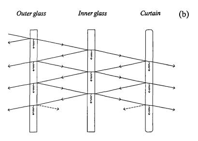
Figure 5.18 Component of transmitted, absorbed and reflected short wave flux (solar beam) incident upon: (a) single glazing with interior curtain, and (b) double glazing with interior curtain.
