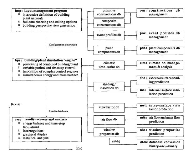
Figure G.1 Program modules of the "ESP" software (series 6, 1990).
