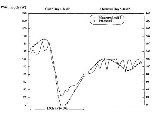
Figure 7.32 Measured and predicted heating requirement of *cell 3* for clear and overcast days. Predicted values are from a simulation run using the "ESP" model.
