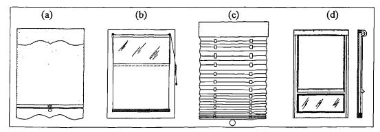
Figure 4.30 Various types of roller shades. (a) common roller shade type; (b) roller shade that rolls up from the bottom with cord and pulley; (c) accordion shade usually made of stiffened polyester fabric drawn with a finger pull; (d) front and side vies of a roller shade on a sealed track to increase its insulation effectiveness. (see Nielson 1990 for more examples).
