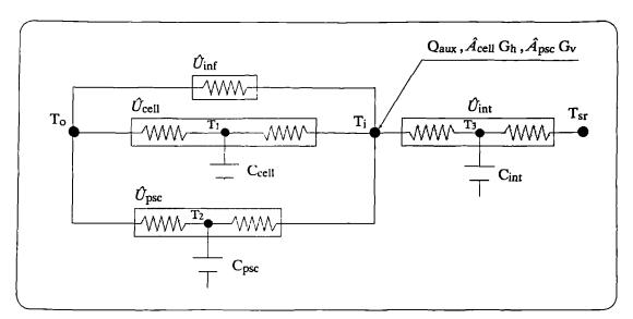
Figure 7.11 Thermal model of the Passys test cell.
