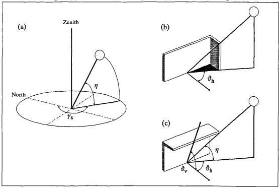
Figure 4.19 An example of graphical determination of solar radiation penetration through a window and a fixed shading device.
