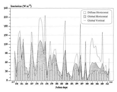
Figure 8.3 Average daily insolation (global horizontal, diffuse horizontal and global insolation on south facing vertical surface) measured at the *Passys* test site for the period from 257 to 313 Julian.
