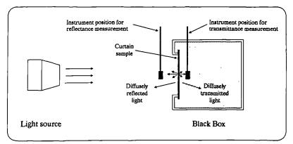
Figure 5.5 Experimental setup for the measurement of transmittance and reflectance of a curtain sample in a dark room. See Figures 5.6, 5.7 and 5.8 for more details.
