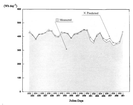
Figure 8.12 Measured and predicted average daily heating requirements of test cell 2 fitted with the curtain. Predicted values are computed by the ESP program for the period from Nov.28th to Dec.27th 1989.
