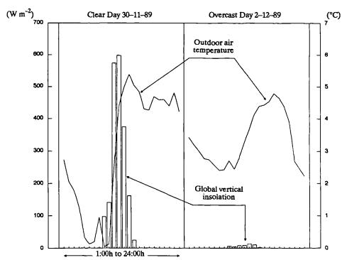
Figure 8.15 Hourly measured global vertical insolation (W m<sup>-2</sup>) and outdoor air temperature (°C) for clear and overcast days from the curtain experiment.
