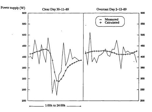
Figure 8.16 Comparison between measured and predicted hourly heating requirements of test cell 2 (with the curtain installed) for clear and overcast days. Calculated data are from the ESP simulation results.
