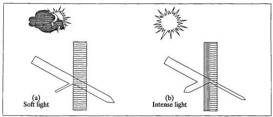
Figure 4.38 Schematic illustration of the polarization mechanism in photo-chromatic glass; (a) matrix in parallel position so light is mostly transmitted; and (b) matrix in crossed position so light is filtered.
