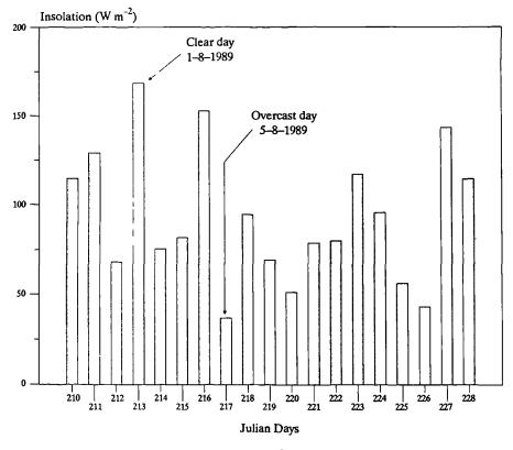
Figure 7.18 Measured global vertical insolation (W m<sup>-2</sup>), for the period from July 29th to August 16th 1989.
