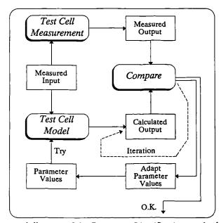
Figure 7.9 Conceptual diagram of the Parameter Identification methodology.
