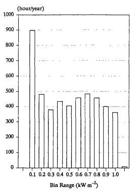
Figure 3.20 Frequency distribution of hourly global horizontal insolation per year of daylight (4767 hours), from the reference climate year of Riyadh.
