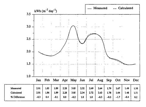
Figure 3.31 A comparison between measured, and calculated monthly mean daily diffuse insolation over the Solar Village, for the year (1986) using monthly regression coefficients of Table 3.12 in Eq.(3.18).
