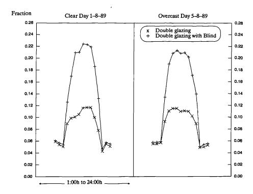
Figure 7.36 Inward-flow fraction  $(N_i)$  of absorbed insolation in the fenestration of *cell 3* and *cell 4* for clear and overcast days. Computed by the "Curtain" program.
