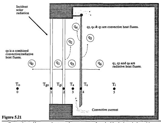
Convective and longwave heat transfer components for a double glazing window with a curtain.
