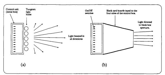
Figure 5.4 Shortwave radiation simulator; (a) the unit beam light in all directions within a hemispherical field; (b) a treatment to direct light to the front side of the black box.
