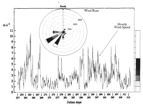
Figure 8.5 Wind speed and direction measured at the *Passys* test site for the period from 257 to 313 Julian. Wind rose represents wind direction frequency with 30° bins, (i.e. -15° to 15°, 15° to 45°, etc).
