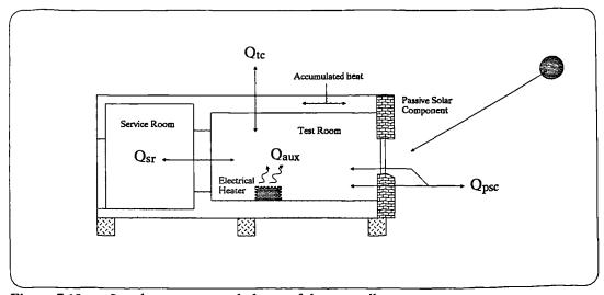
Figure 7.10 Steady-state energy balance of the test cell.
