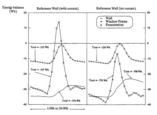
Figure 8.18 Energy balance at the air node of test cell 2 (with and without curtain) due to convective heat exchanges with the reference wall components. Computed by the "ESP" program for a clear day (November 30th 1989).
