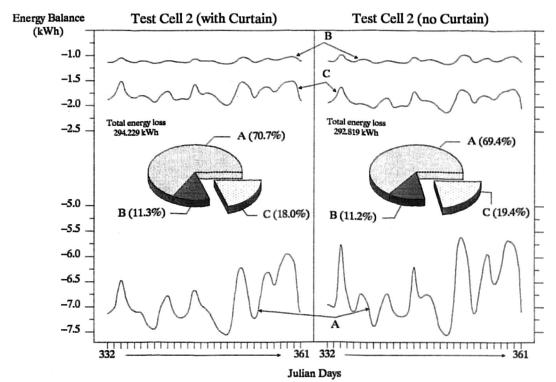
Figure 8.13 Daily total energy balance at the air node of cells 2 (with and without curtain), calculated by the "ESP" model for the period from 332 to 361 Julian. The energy balance at air node is a combination of convective exchanges with (A) the cell side walls, roof and floor, (B) internal wall connecting to the service room, and (C) the passive solar component, i.e. the Reference—wall.
