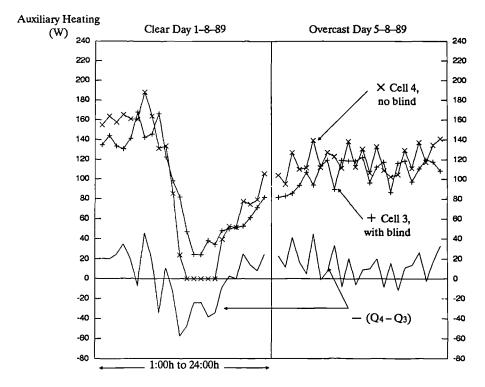
Figure 7.25 Hourly heating requirements of cell 3 and cell 4 (Q<sub>3</sub> and Q<sub>4</sub>) measured for clear and overcast days. Note that the auxiliary heating of cell 4 is modified for the 1.1°C difference in setpoint temperature (see section 7.4.2 for details).
