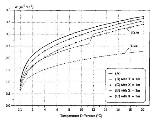
For example, if we consider some vertical surfaces of the heights (X = 1, 1.5, 2, 3 & 4m), using Eq.4.40 & Eq.4.41 with a reference air temperature of 20°C and  $\Delta T = 0.1$  to 20°C, yield the following conditions
