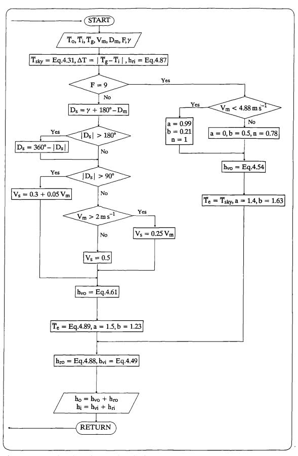
Figure 4.10 Flow chart of HTC Subroutine in QREF.BAS program.
