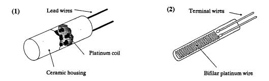
Data sheet DS3 (see Appendix F) describes an RM-Young aspirated thermometer for outdoor temperature measurements. Further characteristics of resistance thermometers are outlined below:
