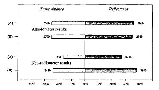
Figure 5.10 Transmittance and reflectance properties of a curtain sample (golden plain weave fabric) as measured by the albedometer and the net-radiometer with two light sources: (A) Tungsten lamp array; (B) Slide projector.
