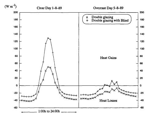
Figure 7.35 Combined convective—longwave heat flux through the fenestration of *cell 3* and *cell 4*. Computed by the "Curtain" program for clear and overcast days.
