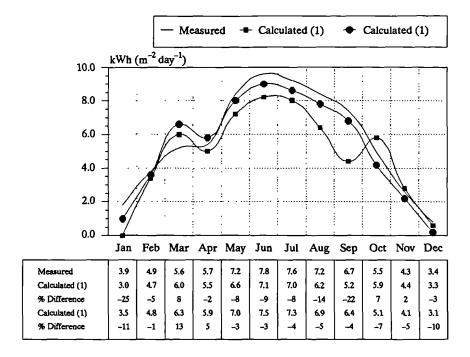
Figure 3.29 A comparison between measured, and calculated monthly mean daily global insolation over the Solar Village, for the year (1986) using the two sets of monthly constants of Table (3.11).
