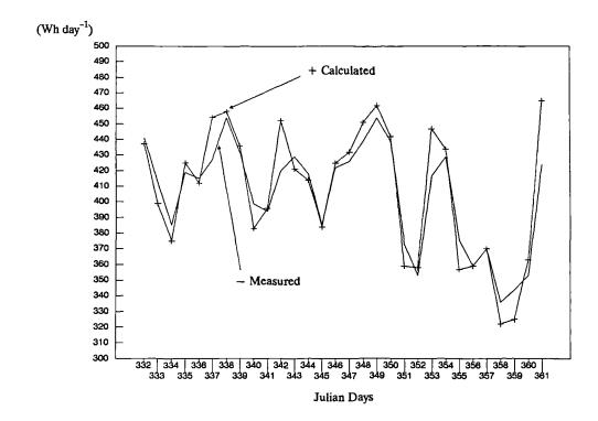
Figure 8.11 Daily average heating requirements of test cell 2 with the curtain installed. A comparison between the measured and calculated values using the regression coefficients derived from the calibration experiment (see Table 8.1).
