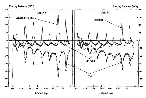
Figure 7.30 Instantaneous energy balance at the air nodes of cells 3 & 4, due to convective exchanges with the test cell components (side walls, roof and floor), timber-frame wall components, and fenestration. Calculated by the "ESP" model for the free floating period of the experiment.
