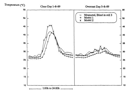
Figure 7.38 Measured and predicted temperature of the *Passys Blind* in *cell 3* for a clear and overcast days. Model 2 refers to results from the "Curtain" program, and model 1 refers to results from the "ESP" simulation run. Note that the ESP predicted values are for the inner layer of the fenestration which include both properties of the glass and the blind (see section 7.5.1 for details).
