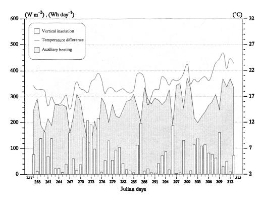
Figure 8.7 Average data (over 24h) of global vertical insolation (W m<sup>-2</sup>), auxiliary heating of the cell (Wh per day), and the difference between the cell ambient and outdoor air temperatures (°C). Measured at the *Passys* test site for the period from 257 to 313 Julian.
