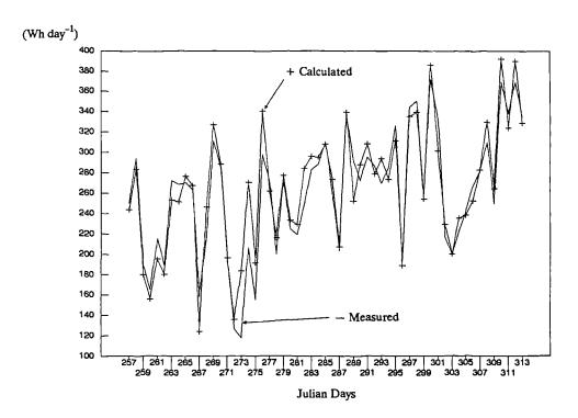
Figure 8.10 Daily average heating requirements of test cell 2 without curtain. A comparison between the measured and calculated values using the regression coefficients derived from the calibration experiment (see Table 8.1).
