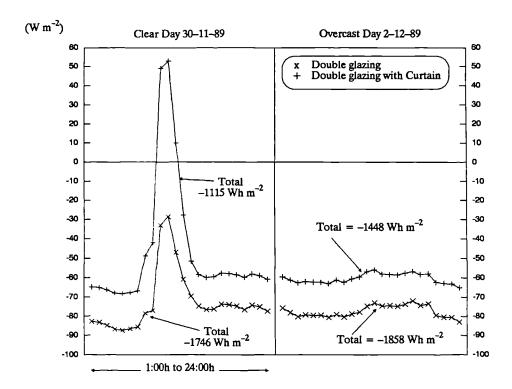
Figure 8.21 Combined convective—longwave heat flux through the fenestration of test cell 2 (with and without curtain). Computed by the "Curtain" program for clear and overcast days.
