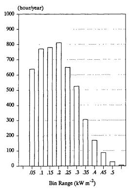
Figure 3.21 Frequency distribution of hourly diffuse horizontal insolation per year of daylight (4767 hours), from the Climate Reference Year of Riyadh.
