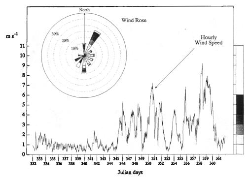
Figure 8.6 Wind speed and direction measured at the test site for the period from 332 to 361 Julian inclusive. (curtain was fitted throughout this period)
