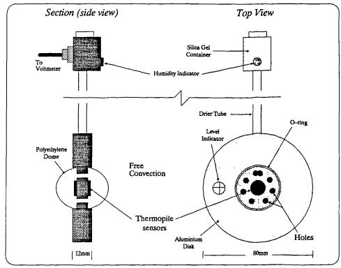
Figure 5.9 A Net-radiometer illustrated in vertical position. The holes allow free air movement between the silica gel container and the thermopile sensors. This will cause noise in the instrument output, particularly in measuring low radiation levels.
