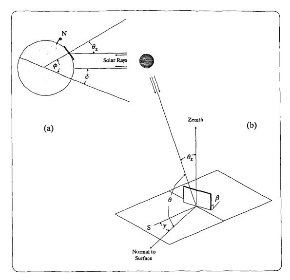
Figure 2.5 Solar geometry. (a) Cross section of earth at solar noon, showing the relationship between latitude  $\phi$ , declination  $\delta$ , and the zenith angle  $\theta_z$ . (b) Angular relationship between a vertical surface and solar beam. The angle of incidence is denoted by  $\theta$ ,  $\beta$  is the surface slope, and  $\gamma$  is the surface azimuth angle.
