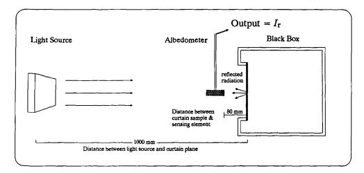
Figure 5.7 Test procedure (second step) to determine the reflectance of a curtain fabric. Note that the first step is typical to that of Figure 5.6. (see text for details).
