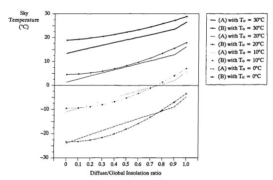
Figure 4.4 Non-clear sky temperature as a function of sky condition, for outdoor air temperatures of 0, 10, 20 & 30°C. Calculated by the author using: (A) Eq.4.38; (B) Eq.4.35. Note that cloud cover factor in Eq.4.35 is taken as  $C = G_{fh}/G_h$ .
