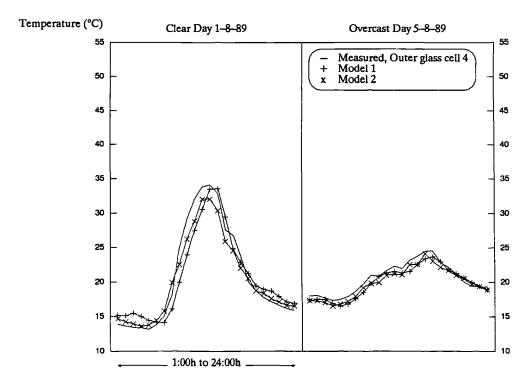
Figure 7.42 Measured and predicted temperature of the *outer glass panel* in *cell 4*, for a clear and overcast days. Model 1 refers to results from the "ESP" simulation run and model 2 refers to results from the "Curtain" program.
