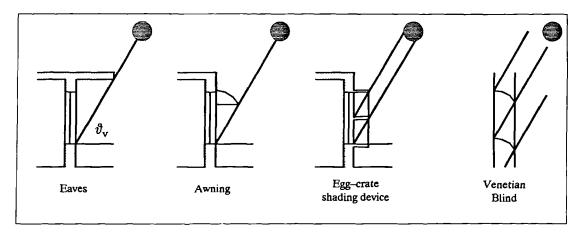
Figure 4.22 Various shading devices for a set performance ( $\vartheta_v = 60^\circ$ ).
