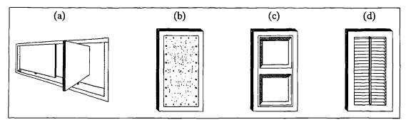
Figure 4.32 Various types of insulating shutters; (a) pivoting shutters, which can be made of plain wood, or fabric-covered wood; (b) rustic riveted wood shutter; (c) raised-panel shutter made of wood or rigid insulation material; and (d) movable-louver shutter. (reproduced from Nielson 1990).
