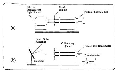
Figure 5.1 Openness factor measuring instruments, (a) arrangement for the visible solar spectrum (0.3–0.7μm) using a photo cell; and (b) arrangement for solar spectrum (0.4–1.15μm) using a silicon cell. (reproduced from Yellott 1965).
