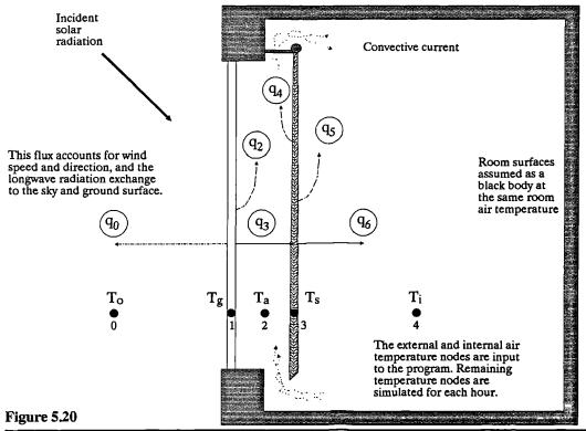
Convective and longwave heat transfer components for a single glazing window with a curtain.
