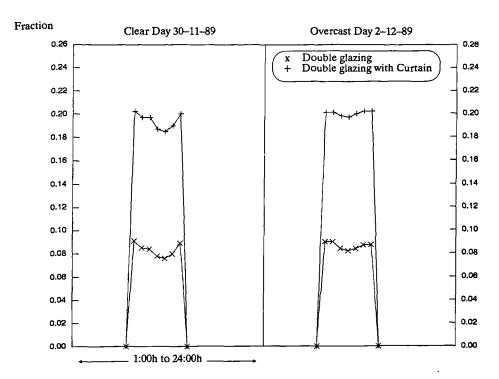
Figure 8.22 Inward-flow fraction  $(N_i)$  of absorbed insolation in the fenestration of test cell 2 (with and without curtain). Computed by the "Curtain" program for clear and overcast days.
