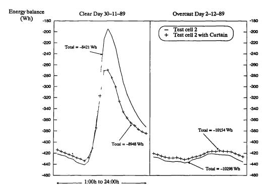
Figure 8.17 Energy balance at the air node of test cell 2 (with and without curtain). Computed by the "ESP" program for clear and overcast days.
