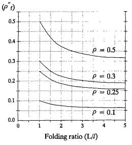
Figure 5.12 Apparent reflectivities  $(\rho^n_f)$  for diffusely reflecting curtain fabrics under diffuse insolation.  $\rho$  = flat material reflectance. (reproduced from Farber et. al. 1963). Note that reflectance decreases with increase in folds.
