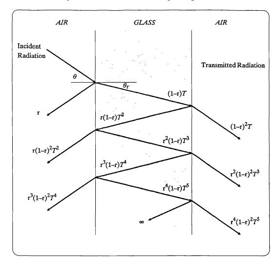
Figure 4.2 Multiple reflection and transmission through a thin glass sheet of finite thickness.
