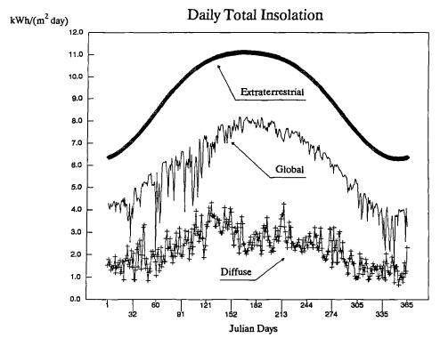
Figure 3.17 Daily global and diffuse solar energy over Riyadh, kWh/(m<sup>2</sup> day), from the Climate Reference Year. Extraterrestrial radiation data are calculated from Eq.3.17 (see section 3.5.1).
