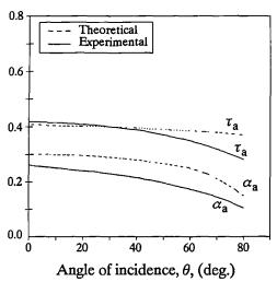
Figure 5.15 Apparent absorptance and transmittance of light coloured curtains ( $\alpha = 0.26$ ;  $\rho = 0.39$ ;  $\tau = 0.35$ ) for 100% fullness and a horizontal shadow angle  $\vartheta_h = 0^\circ$  vs. angle of incidence of solar radiation, for both theoretical and experimental determinations. (reproduced from Farber et. al. 1963).
