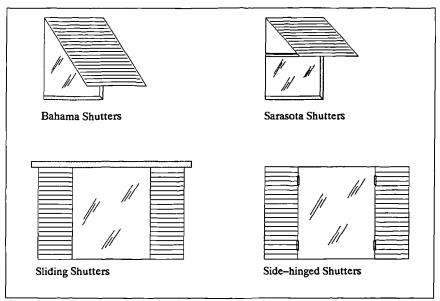
Figure 4.25 Types of exterior shutters.
