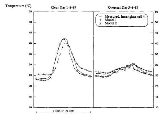
Figure 7.40 Measured and predicted temperature of the inner glass panel in cell 4, for a clear and overcast days. Model 1 refers to results from the "ESP" simulation run and model 2 refers to results from the "Curtain" program.
