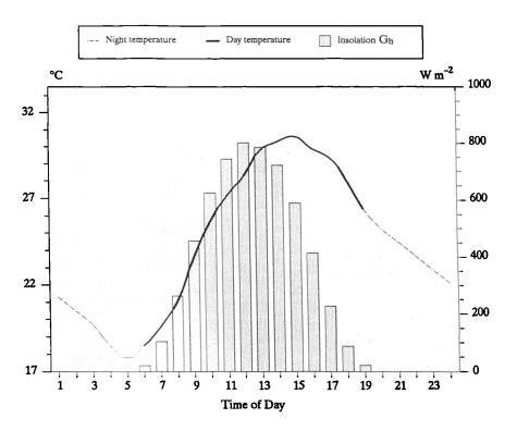
Figure 3.22 Yearly mean of hourly insolation (G<sub>h</sub>) and temperature (Dry Bulb) variations through the day, (from the Climate Reference Year of Riyadh developed in section 3.3).
