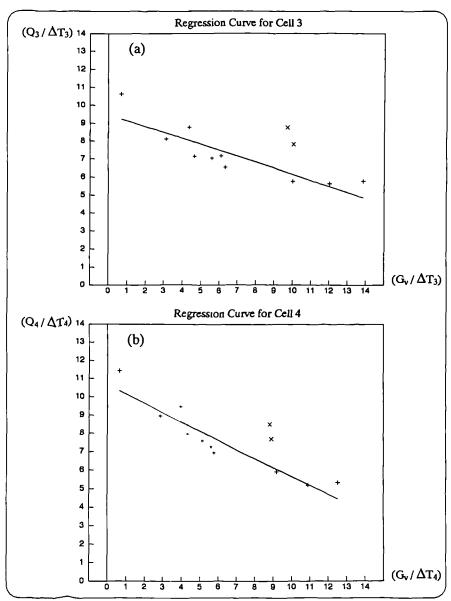
Figure 7.19 Regression curves for (a) cell 3 fitted with glazing and the Passys blind, and (b) cell 4 fitted with glazing only. The two average daily parameters marked "x" have large residual values and correspond to days 210 and 218 Julian.
