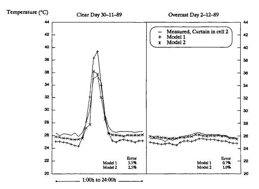
Figure 8.24 Measured and predicted temperature of the curtain, installed in cell 2, for a clear and overcast days. Model 2 refers to results from the "Curtain" program, and model 1 refers to results from "ESP" simulation run. Note that the ESP predicted values are for the inner layer of the fenestration which include both properties of the glass and the curtain.
