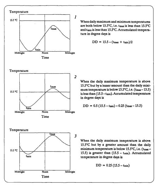
Figure 2.9 Formulae for the calculation of degree days, 15.5°C base, as defined and used by UK Meteorological Offices. (reproduced from the Department of Energy, UK).
