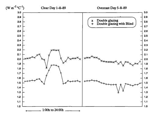
Figure 7.37 U-value of the fenestration in cell 3 and cell 4 for clear and overcast days. Computed by the "Curtain" program.
