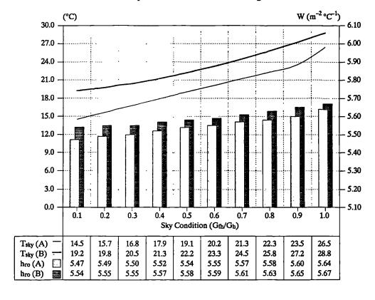
If we assume that the ratio of diffuse to global horizontal insolation is closely related to the cloud cover (i.e.  $C \approx G_{fh}/G_h$ ) then a comparison between Eq.4.35 & Eq.4.38 can be made for different cloud cover factors as shown in Figure (4.4).
