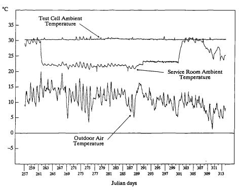
Figure 8.1 Hourly ambient temperatures measured for the period from 257 to 313 Julian. The test cell temperature is taken as the average of air temperatures at 7 locations in the test room, while the service room temperature is taken from one sensor at the centre of the room.
