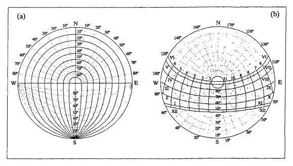
Figure 4.21 Shading design tools. (a) The shading mask protractor to be overlaid on the sun chart. (b) Sun chart for latitude 24°N; it gives the solar azimuth and altitude angles for every time of day and every month (indicated by Roman Numerals I through XII). (reproduced from Givoni 1976).
