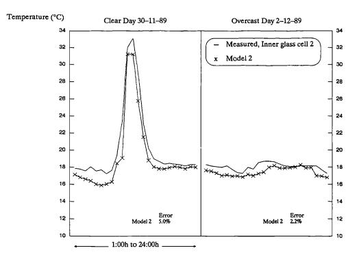
Figure 8.25 Measured and predicted temperature of the *inner glass panel* in *cell 2* with the curtain installed, for a clear and overcast days. Model 2 refers to results from the "Curtain" program.
