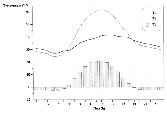
Figure 2.6 Sol-air temperature  $(T_e)$ , at a horizontal roof in July (Riyadh climate) compared with external air temperature  $(T_o)$ . The negative values of the excess sol-air temperature  $T_x$  (which represent the second term in Eq.2.8) means longwave radiation losses to the sky dome at night.
