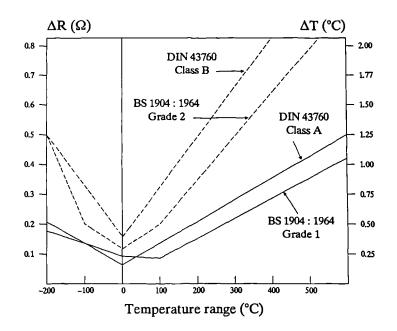
Figure 6.1 Tolerances of British and German Specifications for  $100\Omega$  Thermometers. (reproduced from Labfacility Ltd.)
