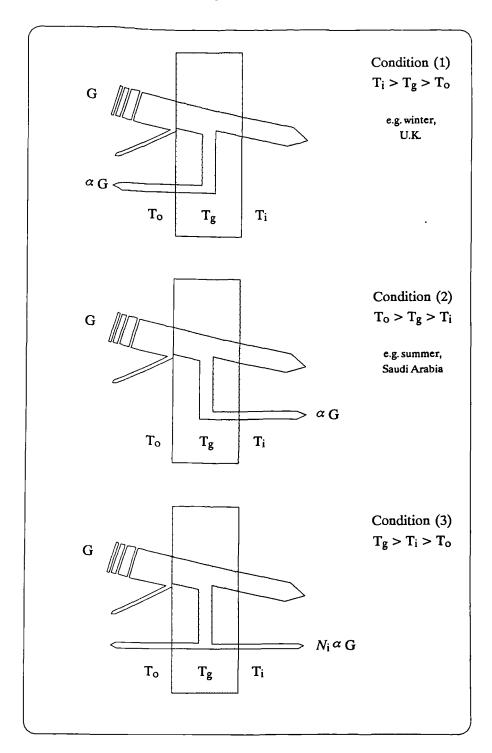
Figure 4.8 Schematic redistribution of absorbed insolation in a single glass for three possible temperature distributions.
