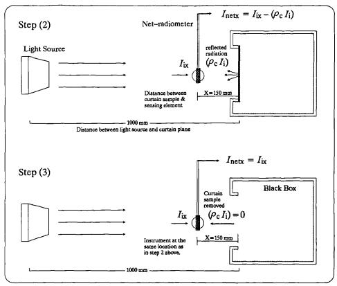
Figure 5.8 Test procedure to determine the reflectance of a curtain fabric using the net-radiometer. Note that the first step is typical to that of Figure 5.6. (see text for details).
