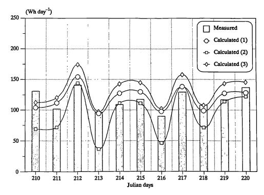
Figure 7.21 Daily average heating requirements of cell 4. A comparison between measured and calculated values using (1) the correlation coefficients for cell 4 in Table 7.11, (2) MRQT output ( $\hat{U}_{tc} = 11.91 \& \hat{A}_{v} = 0.96$ ), and (3) using the correlation coefficients derived from the calibration experiment (see Table 7.9).
