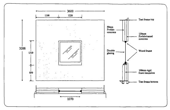
Figure 7.6 Reference wall construction. (elevation, vertical and horizontal sections).
