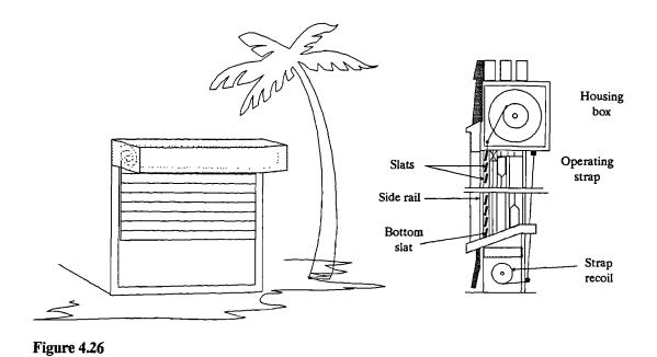
Installation of an external roll blind. (reproduced from Hastings & Crenshaw 1977).
