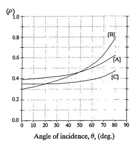
Figure 5.14 Solar reflectance  $(\rho)$  of flat curtain fabrics as a function of incident angle. Type [A] is a light coloured curtain with normal incident properties of  $\tau = 0.35$ ,  $\alpha = 0.26$ ; type [B] a medium coloured curtain with  $\tau = 0.23$ ,  $\alpha = 0.47$ ; and type [C] is a dark coloured curtain with  $\tau = 0.14$ ,  $\alpha = 0.51$ . (reproduced from Farber et. al. 1963).
