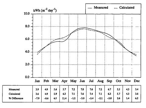
Figure 3.28 A comparison between measured, and calculated monthly mean daily global insolation over the Solar Village, for the year (1986) using the yearly constants (a = 0.42, b = 0.29) in Eq.(3.14).
