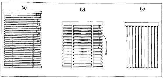
Figure 4.28 Various types of internal blinds. (a) classic miniblind, (b) venetian blind with wide tape and (c) vertical louver blind open and close as curtains and may rotate 180°. (reproduced from Nielson 1990).
