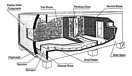
Figure 7.2 Sketch of the PASSYS test cell.
