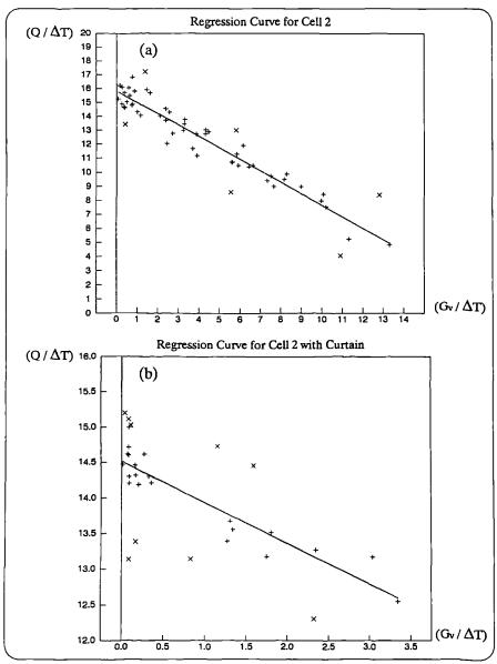
Figure 8.9 Regression curves for (a) cell 2 fitted with glazing only, and (b) cell 2 fitted with glazing and the curtain. The average daily parameters marked "x" have large residual values.
