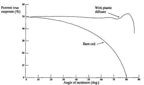
Figure 6.14 Angular response of silicon solar cells with and without a plastic diffusing cover. (reproduced from Coulson 1975)
