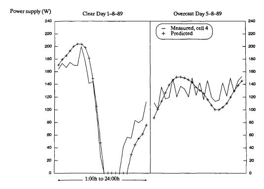
Figure 7.33 Measured and predicted heating requirement of cell 4 for clear and overcast days. Predicted values are from a simulation run using the "ESP" model.
