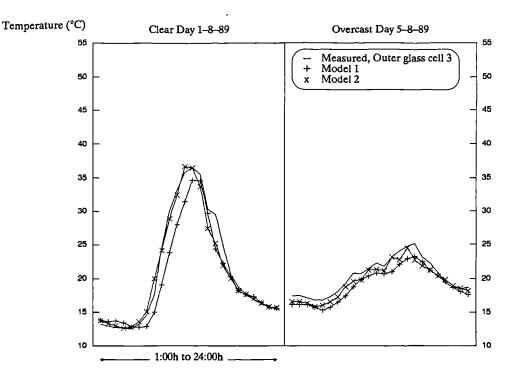
Figure 7.41 Measured and predicted temperature of the *outer glass panel* in *cell 3*, for a clear and overcast days. Model 1 refers to results from the "ESP" simulation run and model 2 refers to results from the "Curtain" program.
