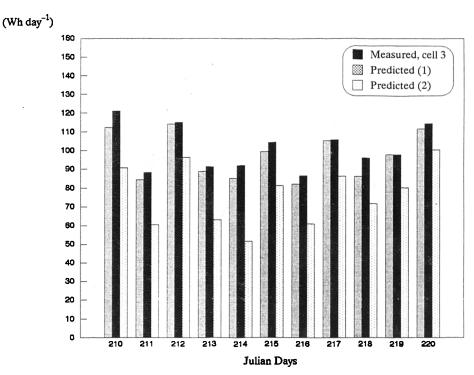
Figure 7.26 Measured and predicted heating requirement of cell 3. Predicted values are from the two "ESP" simulation runs; with the fenestration described as (1) transparent multi-layered construction, and (2) default window with blind control. (see section 7.5.1).
