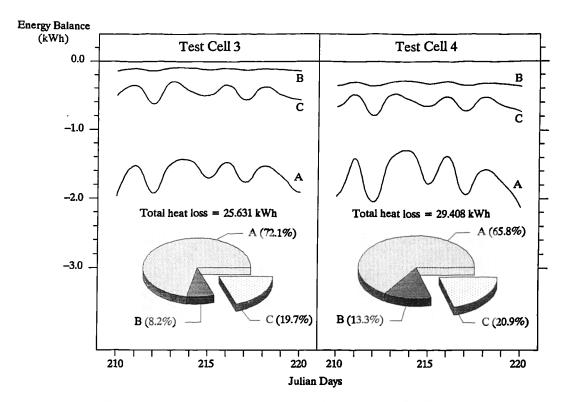
Figure 7.28 Daily totals of the net energy balance at the air nodes of cells 3 & 4, calculated by the "ESP" model for the period from 210 to 220 Julian. The energy balance at air node is a combination of convective exchanges with (A) the cell side walls, roof and floor, (B) internal wall connecting to the service room, and (C) the passive solar component, i.e. the timber-frame wall.
