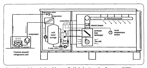
Figure 7.8 Schematic view of the test cell with the heating and cooling system (HCS).
