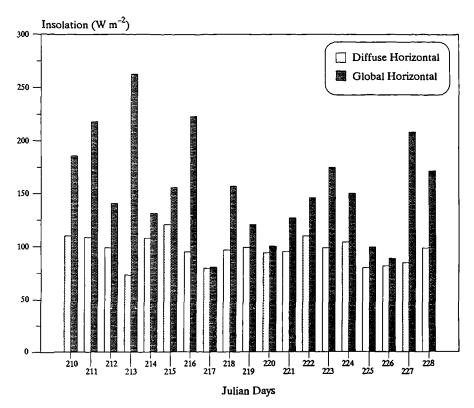
Figure 7.17 Measured global horizontal and diffuse horizontal insolation (W m<sup>-2</sup>), for the period from July 29th to August 16th 1989.
