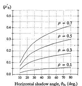
Figure 5.13 Apparent reflectivities  $(\rho_b)$  for direct insolation in diffusely reflecting cavity of the folded curtain.  $\rho$  = flat material reflectance, L/1  $\geq$  2. (reproduced from Farber et. al. 1963).
