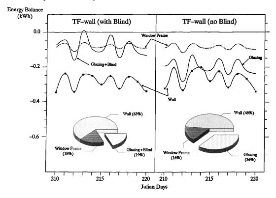
Figure 7.29 A breakdown of the daily total net energy balance at the air nodes of cells 3 & 4, due to convective exchanges with the timber-frame wall components. Calculated by the "ESP" model for the period from 210 to 220 Julian.
