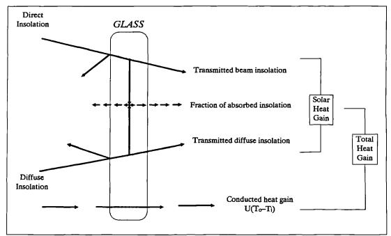
Figure 2.8 Mechanism of heat transfer through glass.
