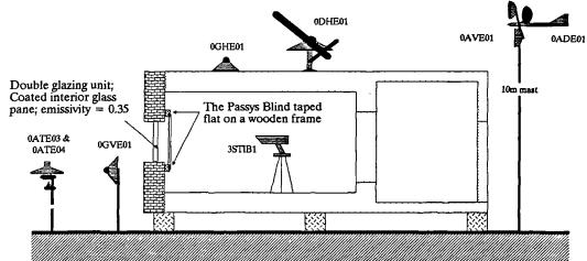
Figure 7.13 A sketch showing the type and location of some basic instruments listed above.
