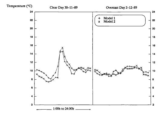
Figure 8.28 Predicted temperature of the outer glass panel in cell 2 without curtain, for a clear and overcast days. Model 1 refers to results from "ESP" simulation run and model 2 refers to results from the "Curtain" program.
