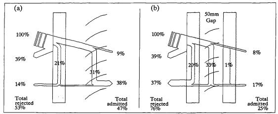
Figure 4.29 Heat transfer mechanism. (a) through a 6mm clear glass with internal light coloured blind; and (b) through double glazing with a blind inside the glazing air gap, which reduces the total transmittance from 72% to 25%. (data from Pilkington 1988; see Table 2.10 in chapter 2 of this thesis for other examples).
