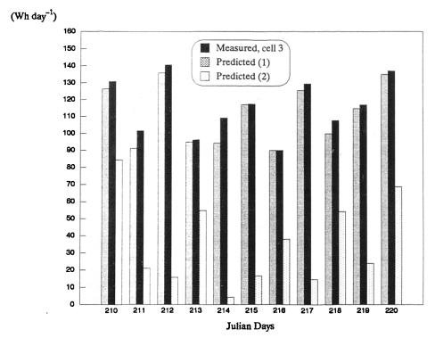
Figure 7.27 Measured and predicted heating requirement of cell 4. Predicted values are from the two "ESP" simulation runs; with the fenestration described as (1) transparent multi-layered construction, and (2) default window with blind control.
