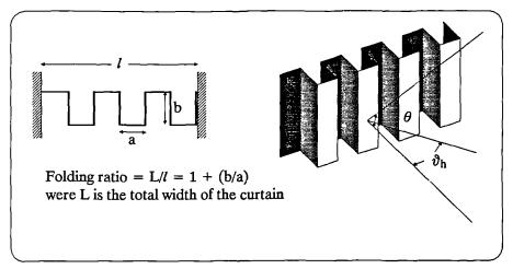
Figure 5.11 Plan and isometric diagrams showing the configuration of a folded curtain for the theoretical analysis of section 5.5.1.
