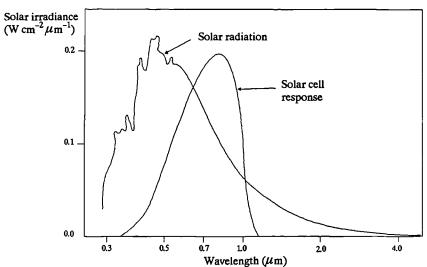
Figure 6.11 Spectral response of silicon solar cells compared with the spectral distribution of solar radiation. (reproduced from Coulson 1975)
