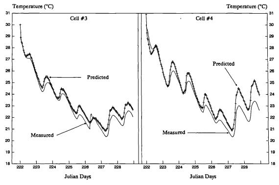
Ambient temperature of cell 3 and cell 4 for the free floating period of the experiment, (August 10th to August 17th 1989). The predicted values are computed by the "ESP" program.
