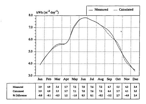
Figure 3.27 Monthly mean daily global insolation over the Solar Village, for the year 1986. A comparison between measured, and calculated values using the monthly constants of Table 3.10 in Eq.(3.14).
