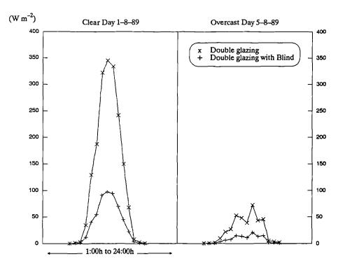
Figure 7.34 Shortwave radiation flux (solar) transmitted through the fenestration of cell 3 and cell 4. Computed by the "Curtain" program for clear and overcast days
