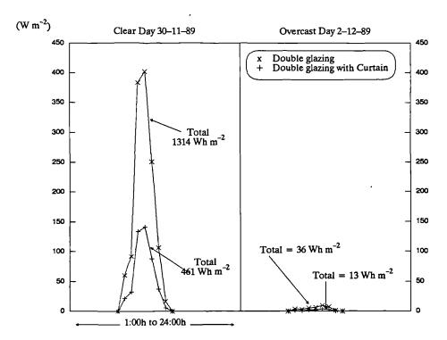
Figure 8.20 Shortwave radiation flux (solar) transmitted through the fenestration of test cell 2 (with and without curtain). Computed by the "Curtain" program for clear and overcast days.
