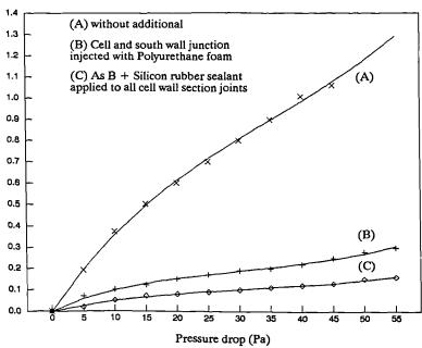
Figure 7.12 Improvements in air tightness of the Passys test cell fitted with the opaque calibration wall. (data from Baker 1990)
