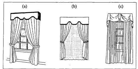
Curtain arrangements for energy efficiency showing; (a) the use of upholstered cornice, made of hard material like plywood in this case, increases the curtain insulative property by trapping an air layer between the glazing and the curtain; (b) the insulative property of curtains is further improved by using liners, i.e. another fabric layer; (c) the cornice can also be made of fabric.
