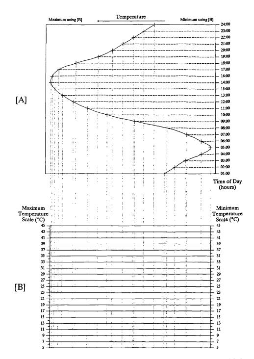
Figure 3.23 Nomogram for predicting diurnal temperature variations in Riyadh. Graph [A] indicates the proportional variations in air temperature during the day. Graph [B] shows the actual variations in temperature which can be related to graph [A], (see section 3.4.1 for instructions).
