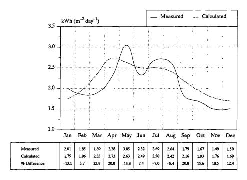
Figure 3.30 Monthly mean daily diffuse horizontal irradiation over the Solar Village, for the year 1986. A comparison between measured, and calculated values using the yearly coefficients (c = 1.061, d = -1.054) in Eq. (3.18).
