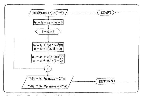
Figure 4.12 Flow chart of GLASS Subroutine in QREF.BAS program.
