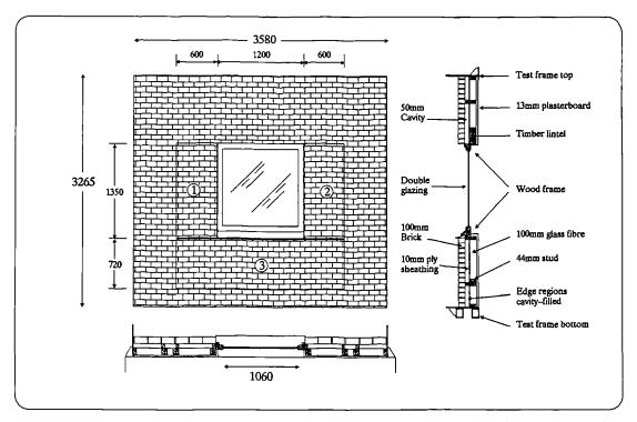
Figure 7.7 Timber-Frame wall construction. (elevation, vertical and horizontal sections). All dimensions in mm. The wall is configurable for different sized windows and patio door by changing the panels numbered 1, 2 and/or 3.
