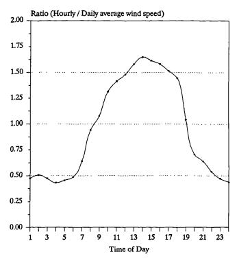
Ratio of hourly to daily average wind speed. If the daily 24h average wind speed is known, multiplying it by the ratio corresponding to an hour on the time—axis gives the wind speed at that time.
