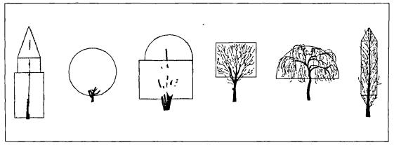
Figure 4.35 Shapes of trees as defined for "SHTREE" program:— spherical, cylindrical, upright cone, reversed cone or any combination of these shapes. (reproduced from Sattler et. al. 1987)
