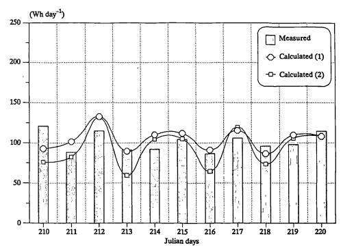
Figure 7.20 Daily average heating requirements of cell 3. A comparison between measured and calculated values using (1) the correlation coefficients  $\hat{U}_{tc} \& \hat{A}_{v}$  derived from the experiment results (see Table 7.11) and (2) using results from MRQT program ( $\hat{U}_{tc} = 10.53 \& \hat{A}_{v} = 0.61$ ).
