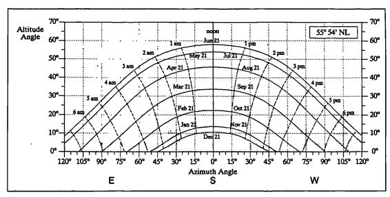
Figure 7.5 Sunchart of the test site. It indicates the shading of the south wall of the test cells by obstructing surfaces as a function of the season and day time.
