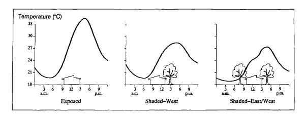
Figure 4.34 Shade tree effectiveness vs. orientation. Temperature scale is in degrees fahrenheit. (reproduced from Hastings & Crenshaw 1977).
