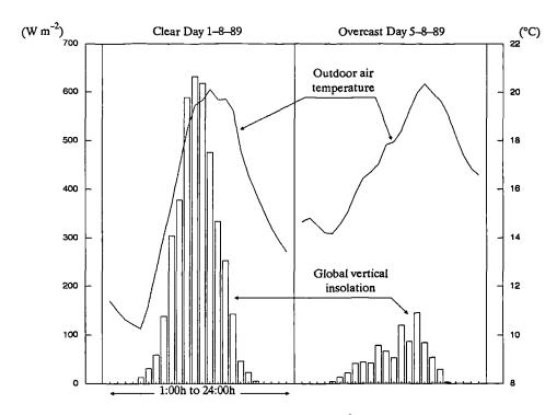
Figure 7.24 Hourly measured global vertical insolation (W m<sup>-2</sup>) and outdoor air temperature (°C) for clear and overcast days.
