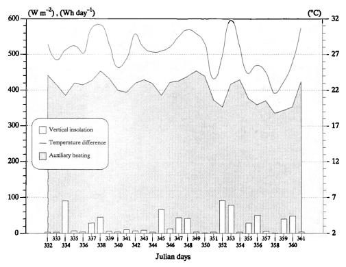
Average data (over 24h) of global vertical insolation (W m<sup>-2</sup>), auxiliary heating of the cell (Wh per day), and the difference between the cell ambient and outdoor air temperatures (°C). Measured at the test site for the period from 332 to 361 Julian with the curtain fitted.
