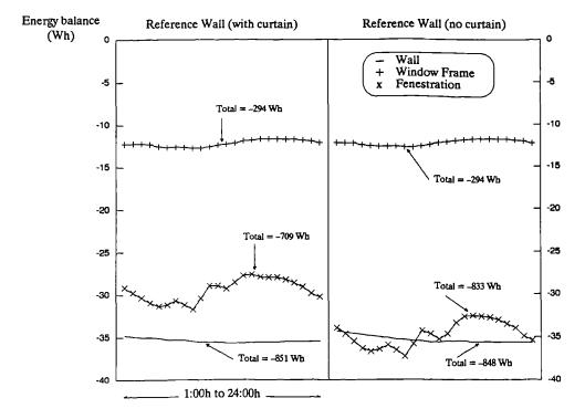
Figure 8.19 Energy balance at the air node of test cell 2 (with and without curtain) due to convective heat exchanges with the reference wall components. Computed by the "ESP" program for an overcast day (December 2nd 1989).
