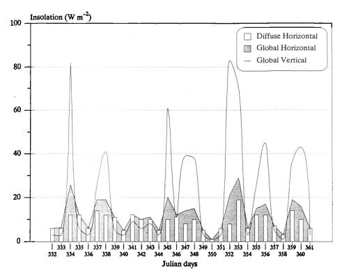
Figure 8.4 Average daily insolation (global horizontal, diffuse horizontal and global insolation on south facing vertical surface) measured at the test site for the period from 332 to 361 Julian.
