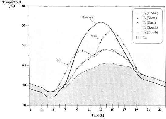
Figure 2.7 Sol-air temperatures at horizontal roof and vertical walls (N, S, E & W orientations) in July (Riyadh climate) compared with external air temperature (T<sub>o</sub>).
