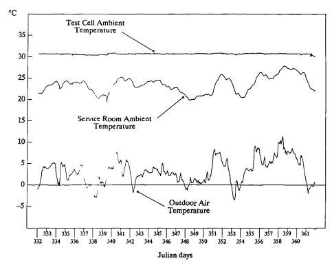
Figure 8.2 Hourly ambient temperatures measured for the period from 332 to 361 Julian inclusive. The curtain was fitted throughout this period.
