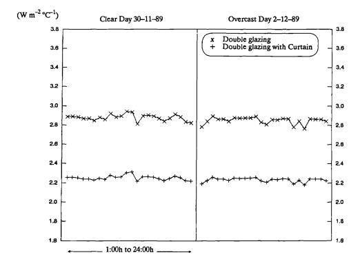
Figure 8.23 U-value of the fenestration in test cell 2 (with and without curtain). Computed by the "Curtain" program for clear and overcast days.
