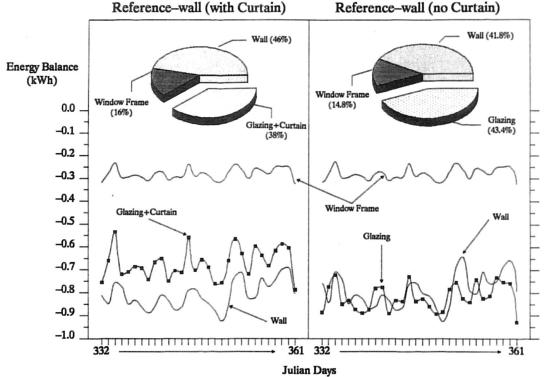
Figure 8.14 A breakdown of the daily total energy balance at the air node of cell 2, due to convective exchanges with the Reference—wall components. Calculated by the "ESP" model for the period from 332 to 361 Julian.
