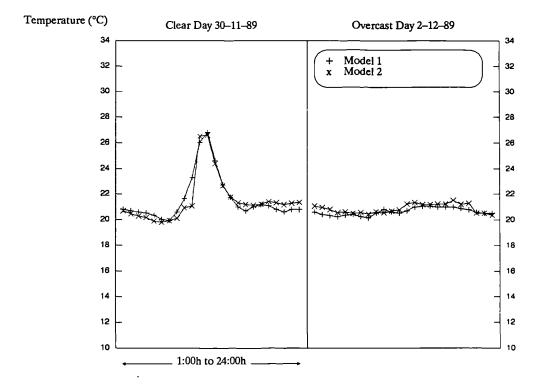
Figure 8.26 Predicted temperature of the *innerglass panel* in *cell 2* without curtain, for a clear and overcast days. Model 1 refers to results from "ESP" simulation run and model 2 refers to results from the "Curtain" program.
