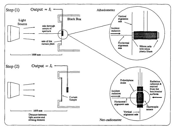
Figure 5.6 Test procedure to determine the transmittance of a curtain fabric. Enlarged diagrams show the alignment of the instrument used.
