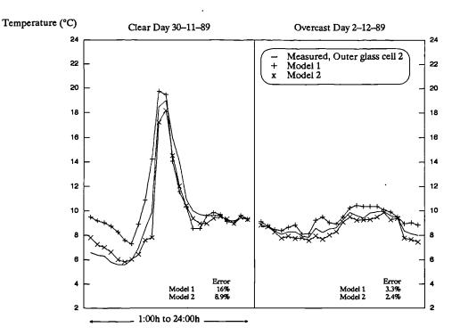
Figure 8.27 Measured and predicted temperature of the *outer glass panel* in *cell* 2 with the curtain installed, for a clear and overcast days. Model 1 refers to results from "ESP" simulation run and model 2 refers to results from the "Curtain" program.
