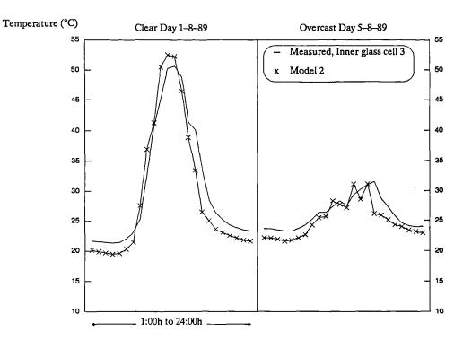
Figure 7.39 Measured and predicted temperature of the inner glass panel in cell 3, for a clear and overcast days. Model 2 refers to results from the "Curtain" program.
