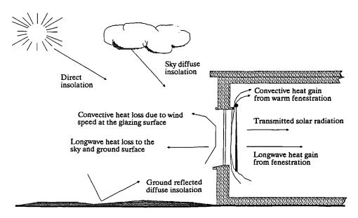
Figure 5.17 Sources of incident solar radiation and components of heat gain/loss through a curtain-shaded window.
