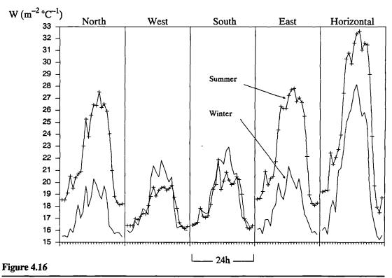
Hourly heat transfer coefficients at the external surface of the reference glass for the stated orientations, W ( $m^{-2}$  °C<sup>-1</sup>). Calculated using Riyadh climatic data (see section 4.4.2).
