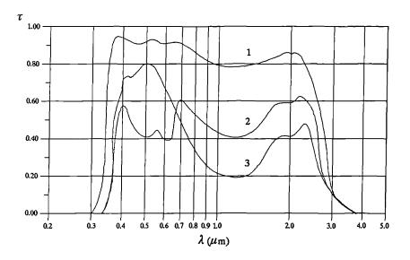
Figure 4.1 Solar spectral transmittance for typical architectural glass. (reproduced from Brunello & Zecchin 1987).
