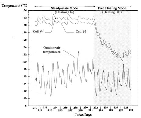
Ambient temperatures measured for the period of experiment. Test cell temperature is taken as the average of air temperatures at 7 locations in the test room (see Table 7.10).
