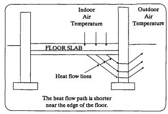
Figure 2.2 Heat flow through floor slab.
