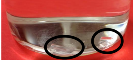
Figure 4. 11 Image of crystals formed when solution was not sheared in the Couette cell.
