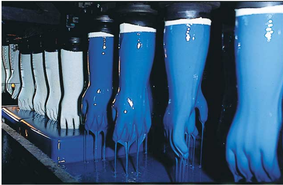
Figure 1.2: Image showing gloves removed from a tank during the dip coating process [1]. (Reproduced with permission.)
