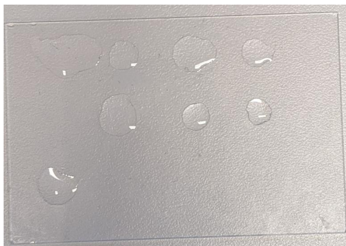
Figure 3-25. Glass slide showing deposited agarose droplets, with non-uniform sizes and points with an absence of agarose, caused by temperature-related nozzle blockage issues.
