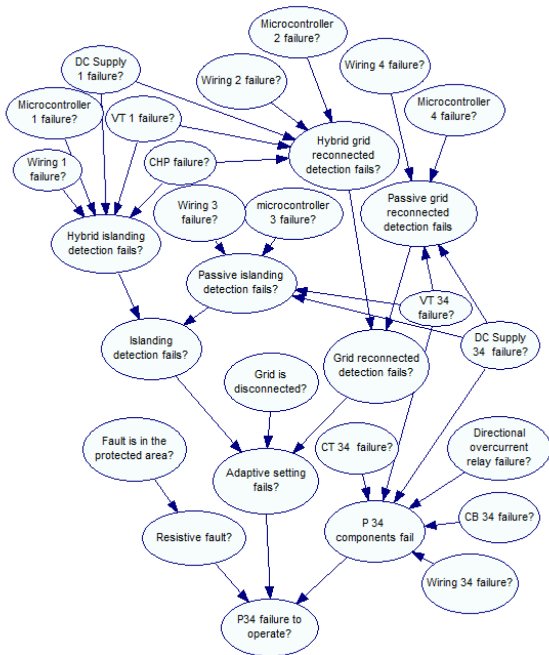
Figure 7.5. Model of protection 34 failure to operate
