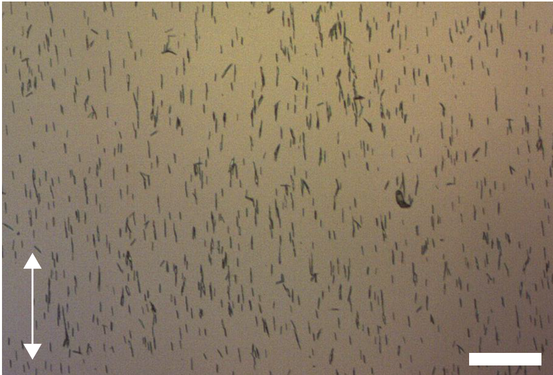
Figure 6.2: Optical micrograph of the fabricated large-scale area on a quartz disk substrate. Arrows indicate the target orientation of the \sim 10 \mu\text{m} NW devices. Scale bar: 100 \mu\text{m} .
