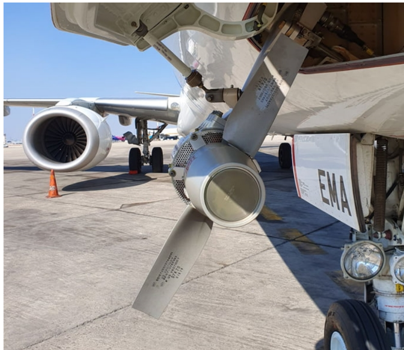
Figure 2-37. RAT on modern aircraft (9GAG, 2019)
