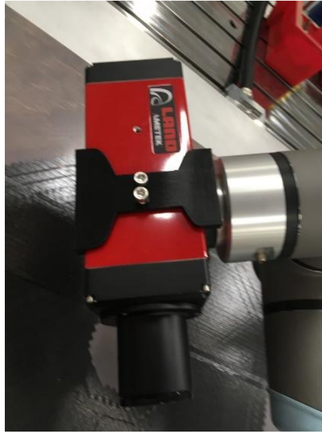
Figure 4.4 – Thermal Camera Mounted on Cobot Using Custom Adapter
