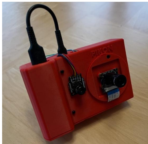
Figure 4.1 – Initial Thermal Imaging Development System Front View
