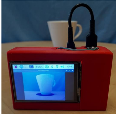
Figure 4.2 – Initial Thermal Imaging Development System Back View
