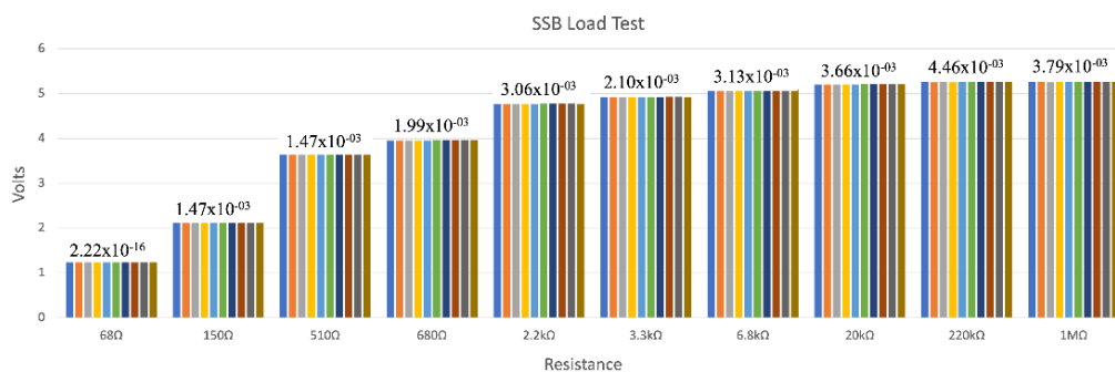
Figure 3.5 – Resistance and Load Testing Results with Standard Deviation Values
