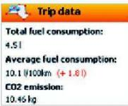
Take control of your carbon footprint with ecoPLUS. The device calculates CO<sub>2</sub> emissions based on your vehicle's engine details and feeds this information back to WEBFLEET. There you can benchmark one or more vehicles using a daily, weekly or monthly parameter to view and compare CO<sub>2</sub> emissions.
