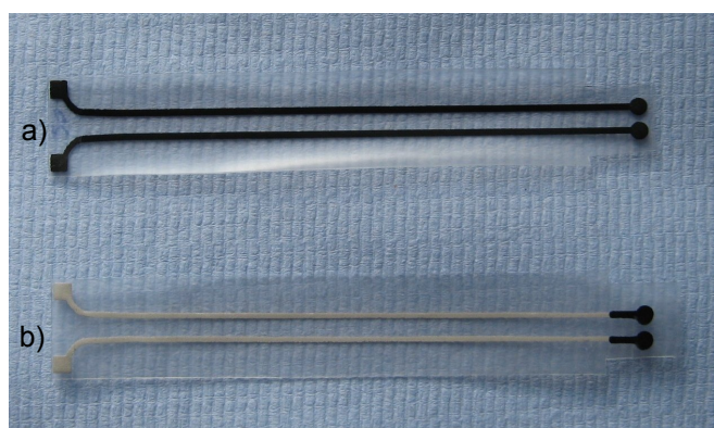
Figure 4-1. The screen-printed sensors used in the carbon preconditioning experiments: a) Carbon on PE300 (C-PE300); b) Carbon tipped on PE300 (C-tip-PE300).
