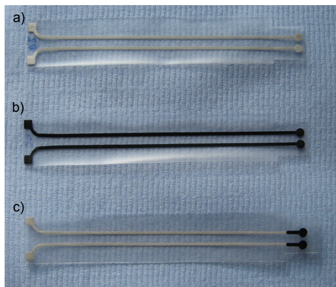
Figure 2-3. The screen-printed electrodes on polyethylene substrate: a) Ag-AgCl; b) Carbon; c) Carbon tipped with a silver track.
