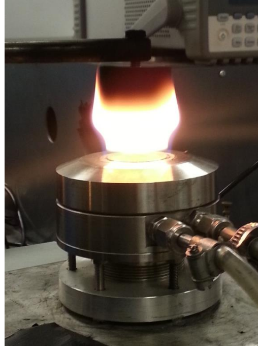
Figure 3-4: Ethylene:air premixed flame \Phi = 2.1
