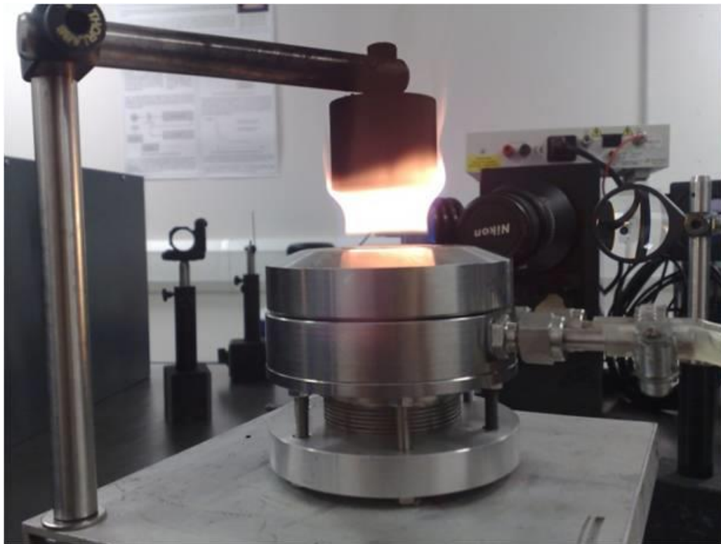
Figure 4-5 : Flame where \Phi = 2.1 . In orange region soot is present
