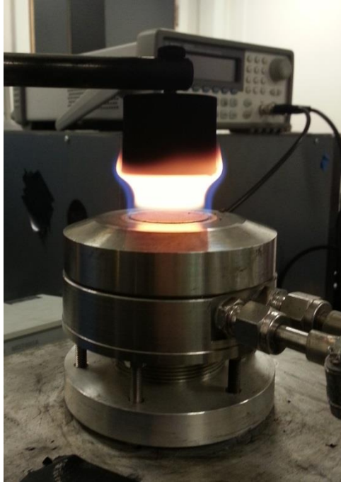
Figure 3-3: Ethylene:air premixed flame \Phi = 1.7
