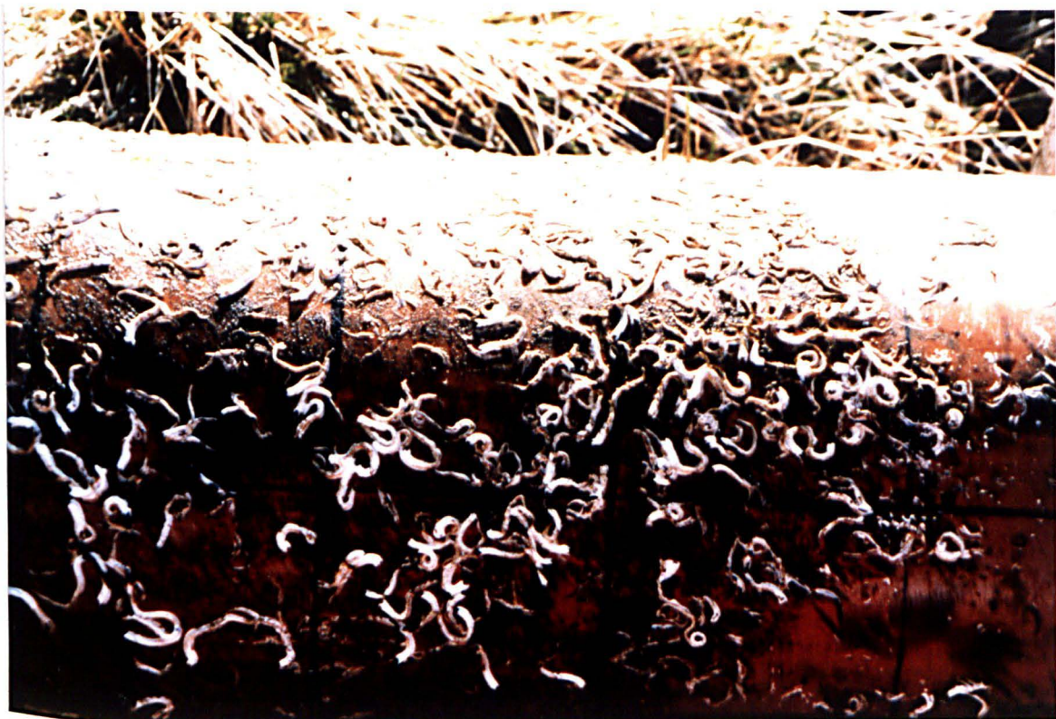
Fig. A.8. Pomatoceros (tubeworm) on a test cylinder at Loch Sween, West Coast of Scotland.
