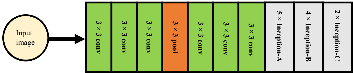
Figure A.5: The Inception-v3 architecture. Adapted from [25].
