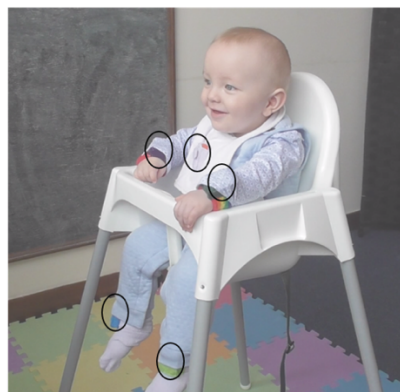
Figure 9-1. Placement of 5 IMUs on infant's body. Black ovals mark the location of sensors hidden in infant clothing
