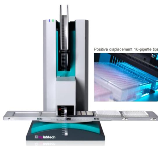
**Figure 133:** Mosquito Liquid handling robot, featuring a 16-pipette tip changeable head, allowing for positive displacement into entire columns of 384-well plates in one dispense with rapid tip exchange. Disposable pipette tips are held in a spool reel of 36,000 tips. Plate deck allows 5 plates (96/384/1536-wells supported) to be positioned on the robot at once. TTPLabTech®.
