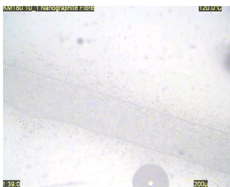
Figure 7-58– 0.1 % Nanographite fibre dissolution
