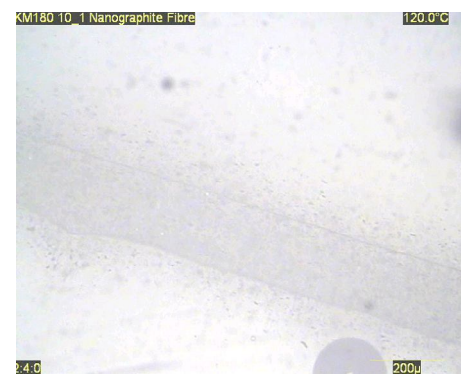
Figure 7-58– 0.1 % Nanographite fibre dissolution
