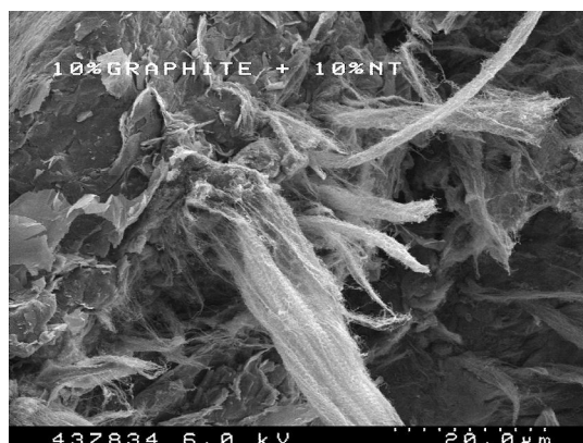
Figure 7-45 – SEM images of 10 % nanographite blended with 10 % nanotubes
