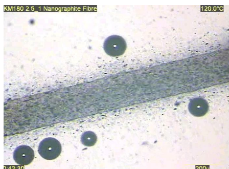
Figure 7-58– 0.1 % Nanographite fibre dissolution
