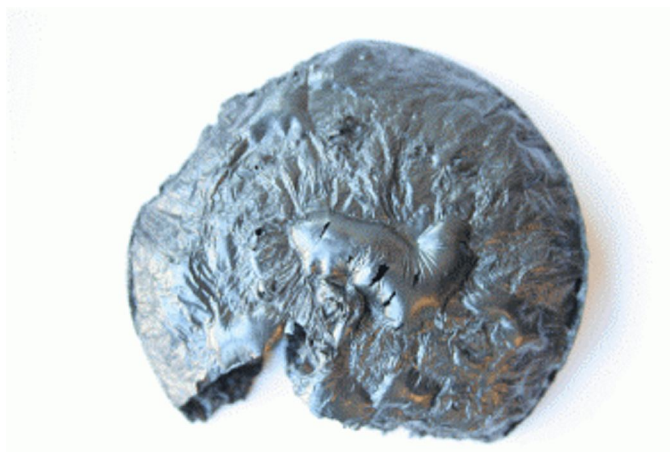
Figure 7-9 – Picture of graphite composite after exposure to vacuum overnight
