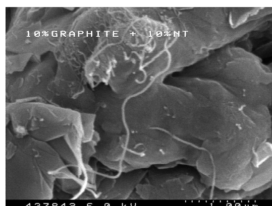
Figure 7-47 - SEM images of 10 % nanographite blended with 10 % nanotubes
