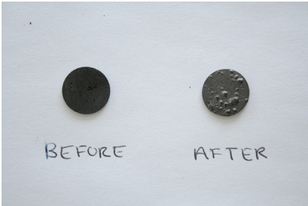
Figure 7-25 – 10 % nanographite + 20 % TTF TCNQ before and after exposure to oven at 240°C
