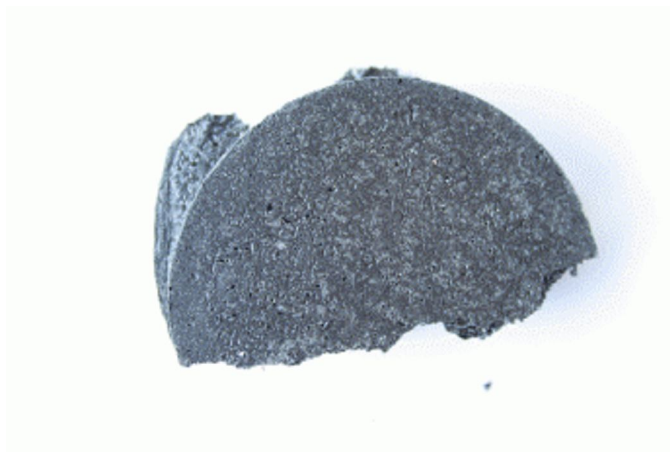
Figure 7-10– Picture of the bottom of 2 % graphite / PES-based co-polymer composite
