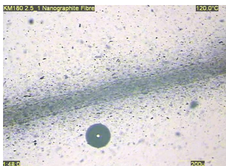
Figure 7-59 - 0.4 % Nanographite fibre dissolution
