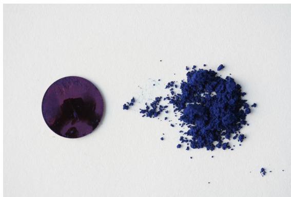
Figure 7-19 – Picture of Cu phthalocyanine in powder and disc form
