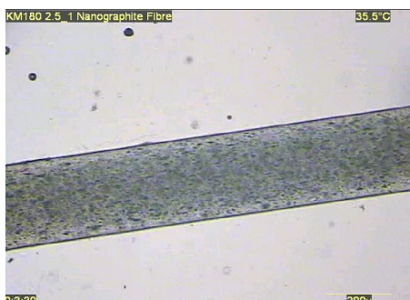
Figure 7-58– 0.1 % Nanographite fibre dissolution
