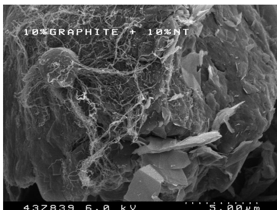
Figure 7-47 - SEM images of 10 % nanographite blended with 10 % nanotubes
