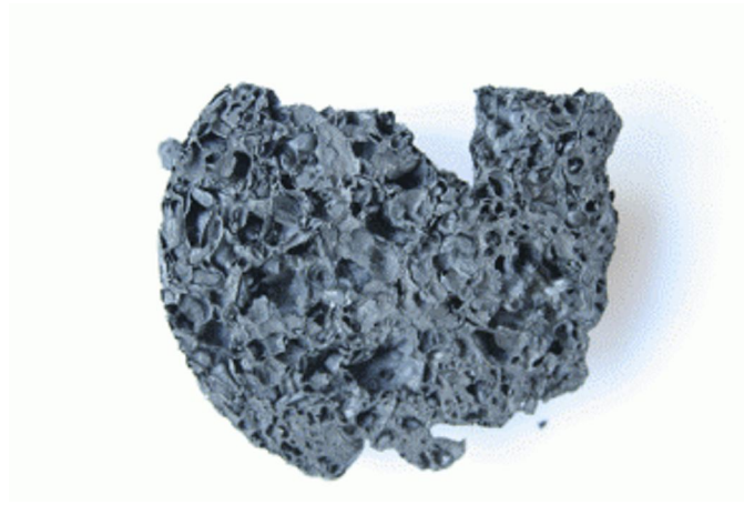
Figure 7-11 – Picture of the bottom of the 80 % graphite / PES-based co-polymer composite
