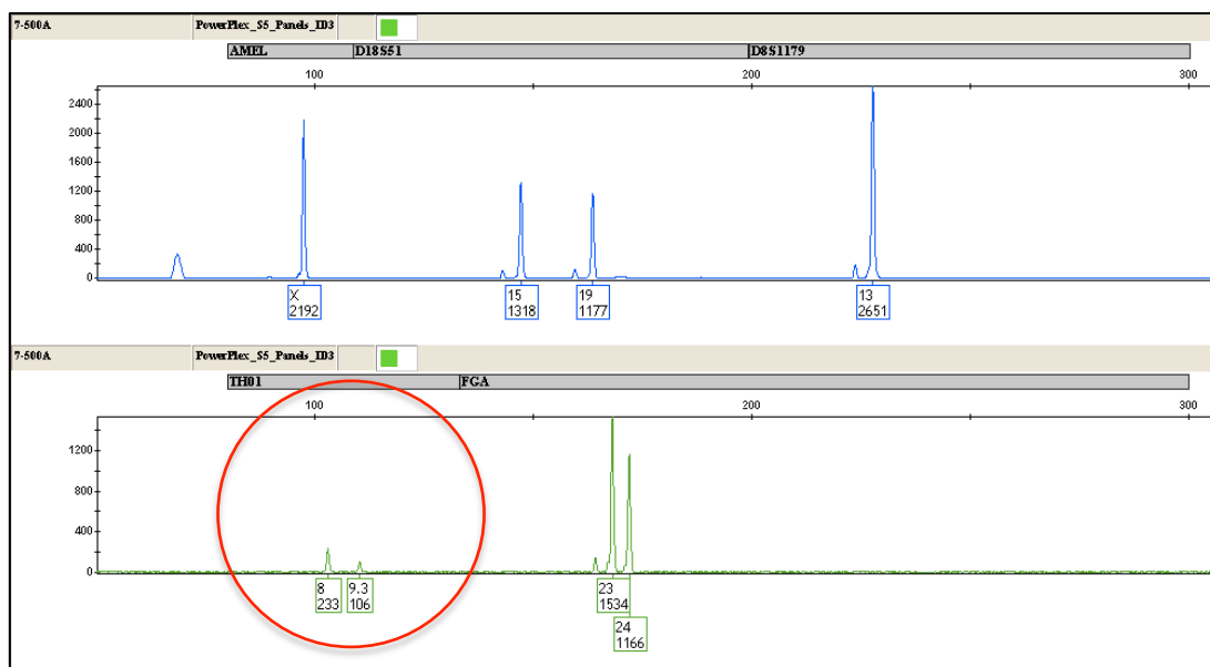
Figure 3.1. EPG of 9947A amplified with S5. Note the peak height of allele 8 and 9.3 (<250 RFUs) for TH01 (circled) while other alleles are above 1000 RFUs.
