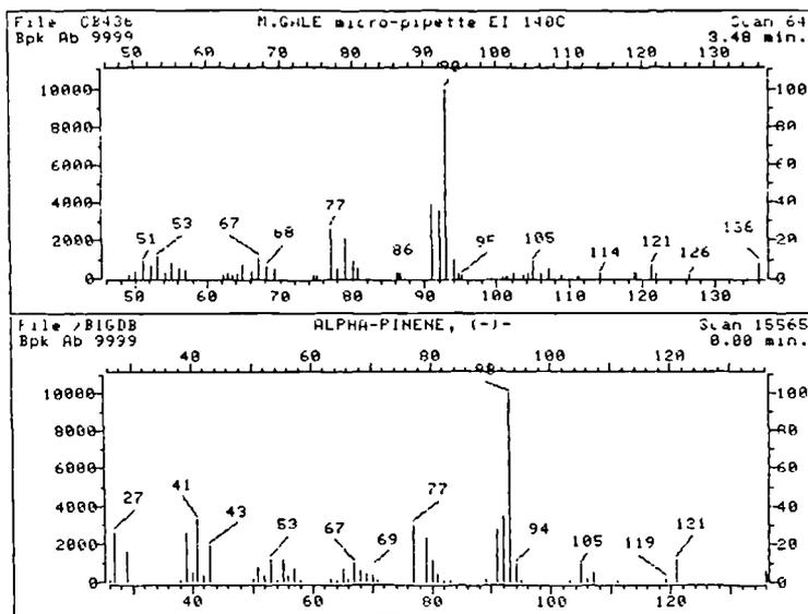
Figure 4.4 A GC-MS comparison of a peak spectrum with a library spectrum of  $\alpha$ -pinene.
