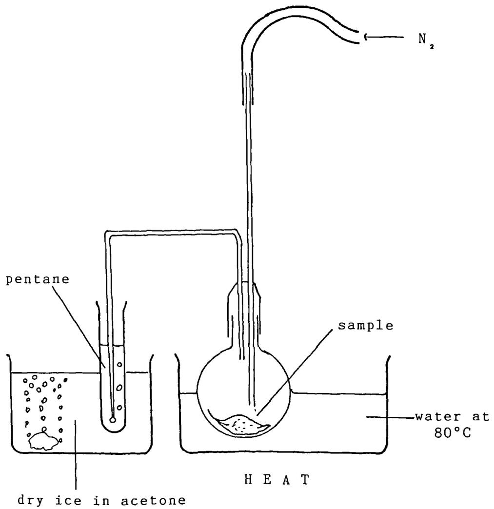
Figure 4.2 Apparatus for extraction of volatile oils from small leaf samples.
