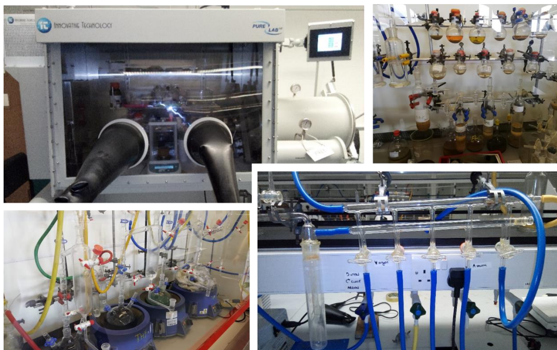
Figure 1.1 – Example inert atmosphere equipment: glovebox, dried reagents/solvent, and Schlenk line.
