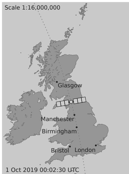
Figure 4.1: Visualisation of the prototype of the national SatQKD communication system. It consists of five optical ground stations spread across the UK. Communication between ground stations is encrypted with symmetric key pairs distributed via a satellite placed into a Sun-Synchronous Orbit. The satellite passes over the UK mainland territory towards the North direction around local midnight. The dashed arc denotes the ground track the spacecraft follows.
