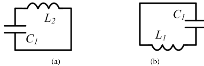
Fig. 3-9. Equivalent model of the power path for the inner capacitor C_1 of the ACVD converter: (a) S_2 is on, S_1 is off and (b) S_1 is on, S_2 is off.
