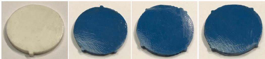
**Figure 105 - Assembled parallel void samples: two cylindrical voids, three cylindrical voids, four cylindrical voids and five cylindrical voids**
