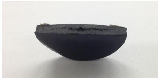
**Figure 118 - Aging cycle three thermally aged sample A at 99.4 deg for 168 hours cross sectional view**
