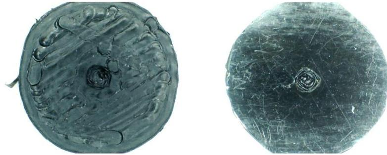
**Figure 90 - 2 mm spherical void in two halves (a) lower half (b) upper half**
