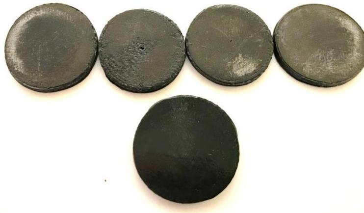
**Figure 120 - Aging cycle seven the four samples subjected to thermal aging (upper) unaged sample (lower)**
