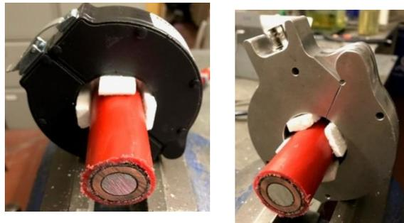
**Figure 23 - 100/50 HFCTs with 11 kV Prysmian EPR cable HDPE casing (left) and aluminium casing (right)**
