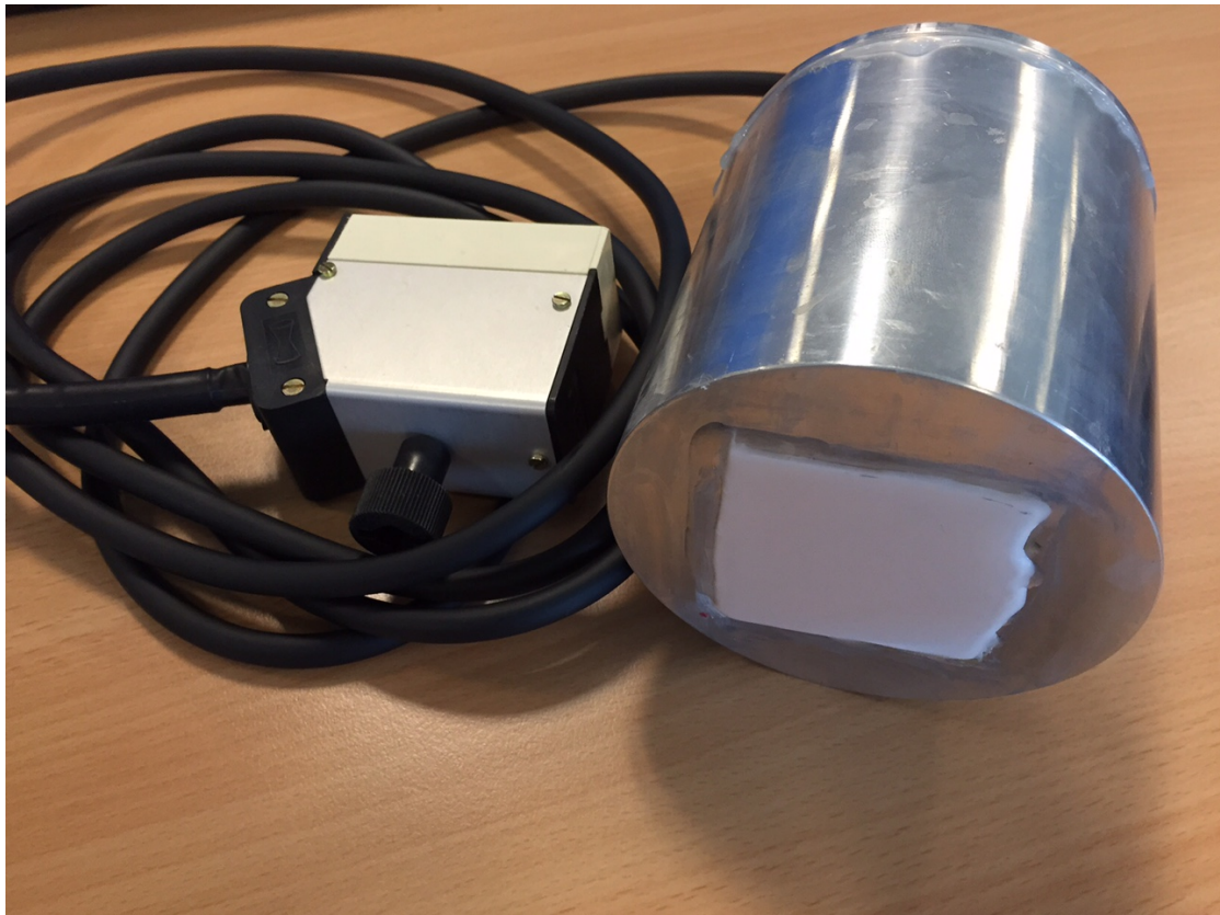
FIGURE 5.14: Photograph of the prototype array in the probe housing with a Hypertronics cable attached.
