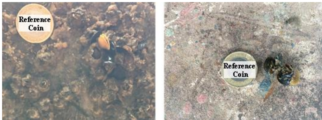
Figure 3-20: Pictures of a barnacle before and after the adhesion strength measurement test
