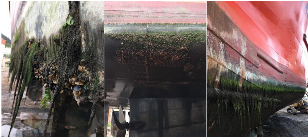
Figure 3-18: Biofouling Accumulation on Various Hull Sections for UW1 Fishing Vessel
