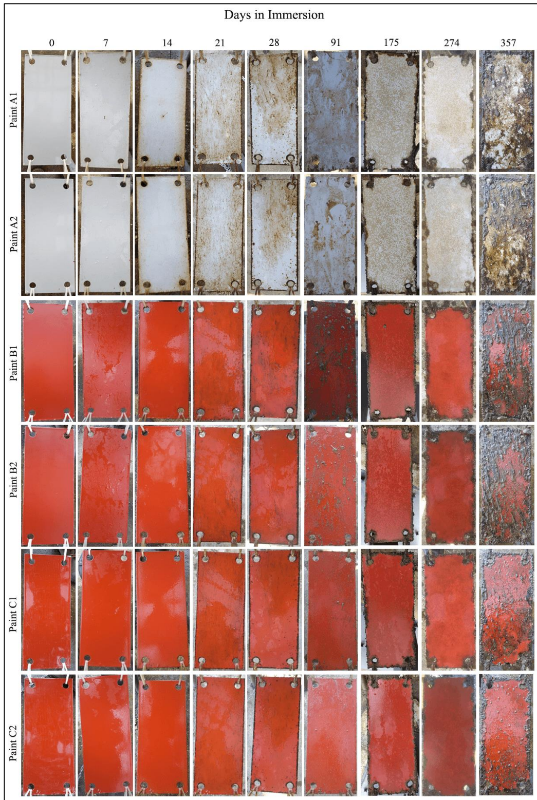
Figure 4-15: FR Immersion test panels' accumulation results in the first 4 weeks, and then 3 months, 6 months, 9 months, and 12 months, respectively.
