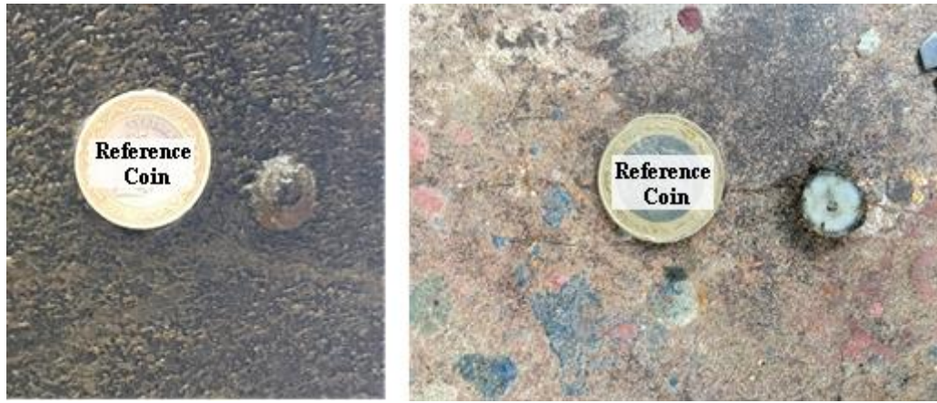
Figure 3-19: Pictures of a barnacle before and after the adhesion strength measurement test
