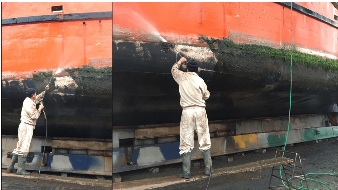
Figure 2-10: Biofouling cleaning process after a year of fishing operation in dry-dock
