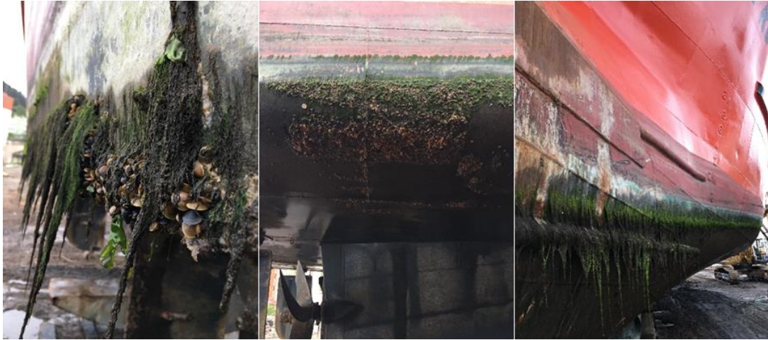
Figure 2-9: Heavy growth of macrofouling after a year of fishing operation on a trawler.
