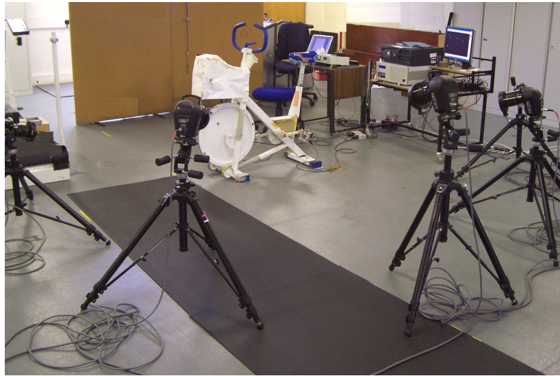
Figure 2.4 Experimental set up using motion analysis.
