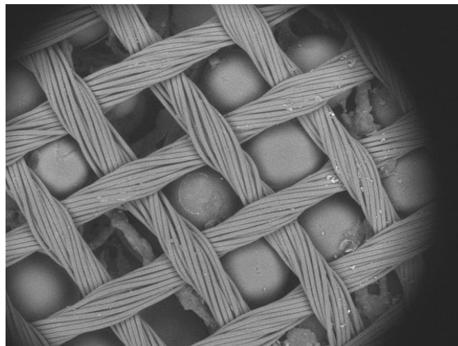
Figure 44: Scanning Electron Microscope (SEM) image of adsorbent beads trapped within suspension membrane
