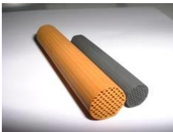
Figure 37: Polymer precursor which undergoes a process of carbonisation which results in a material with a porous structure which can be tightly controlled and tailored to the requirements of the material. Pre-carbonisation on the left and post-carbonisation on the right, note the significant shrinkage involved
