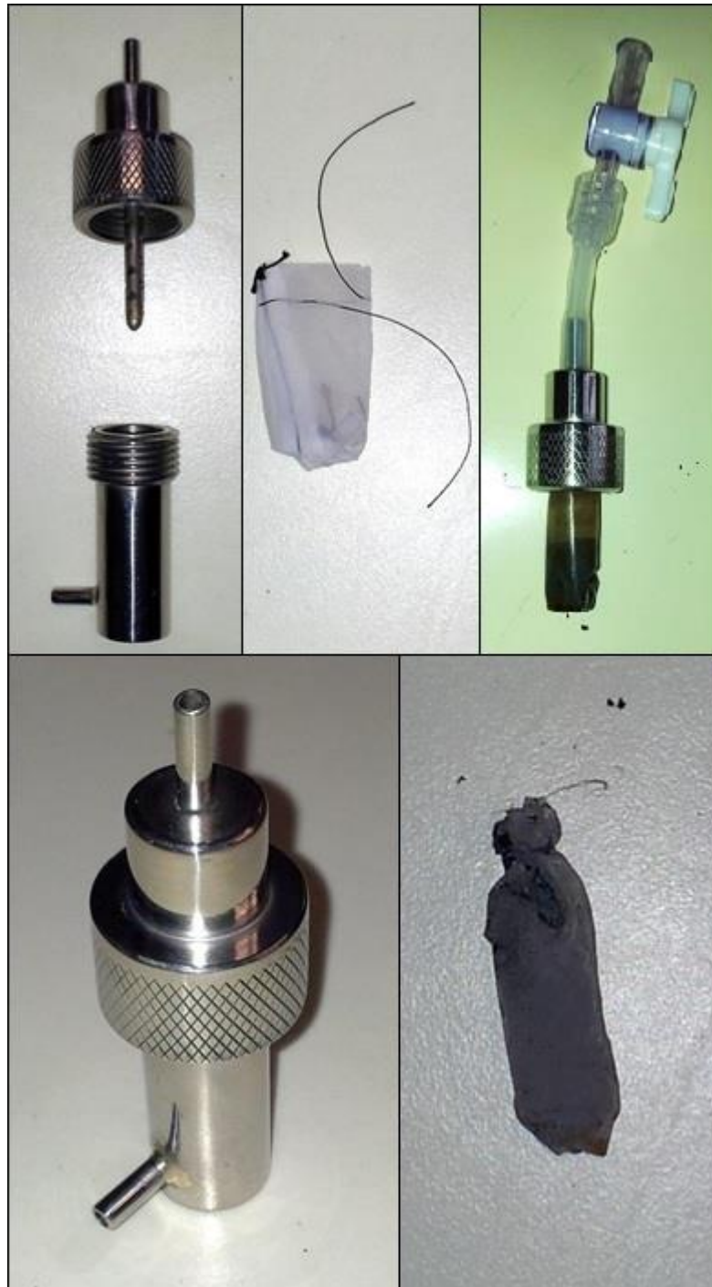
Figure 45: Clockwise from upper left, adsorbent column ready to be loaded with adsorbent, empty "tea bag" ready to be filled and secured to column spindle with surgical thread, loaded adsorbent "tea bag" primed with heparinised saline, assembled adsorbent column, full adsorbent "tea bag" following experimentation.
