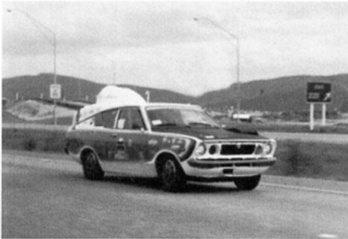
Fig. 2.4 The hydrogen engine car road test by Furuhami et al. [121] in 1975.
