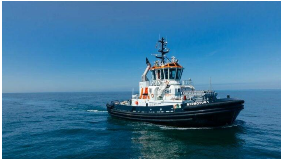
Fig. 2.2 The world’s first hydrogen engine powered tugboat “Hydrotug 1” [87].
