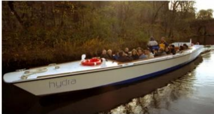
Fig. 2.1 The world’s first hydrogen-powered ship “Hydra” [86].
