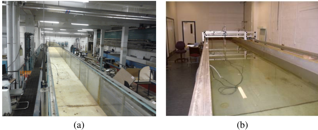
Figure 4.3: Examples of tank tests facilities: a) Flume Tank and b) Tow tank.
