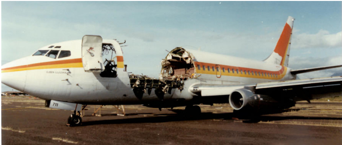
Figure 2.9: Image showing fuselage damage caused to Aloha Airlines flight 243 as a result of fatigue failure [53]
