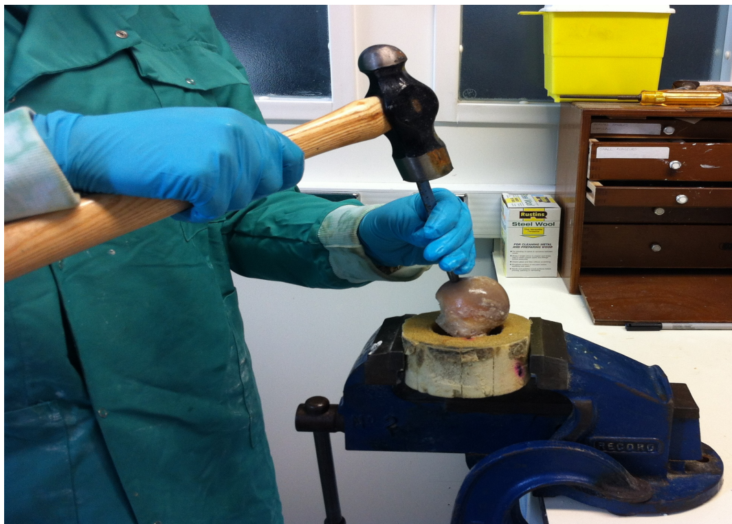
Figure 5.5: 22 plugs were taken from across each femoral head using a tissue punch.
