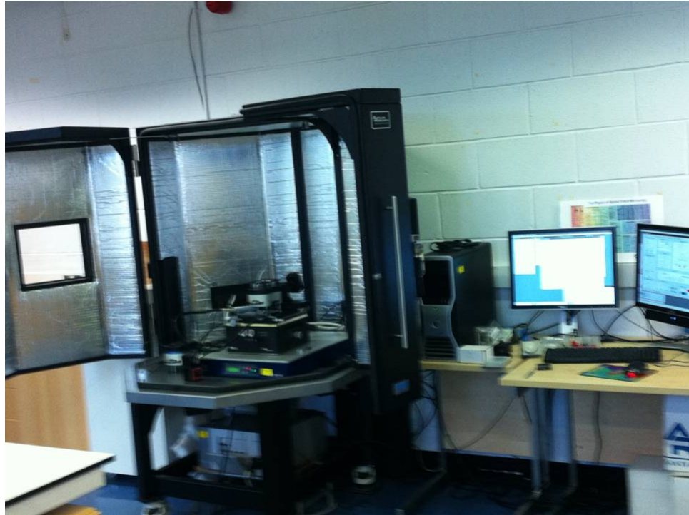
Figure 3.1: Photograph of the whole system with the MFP-3D Nanoindenter head in place.
