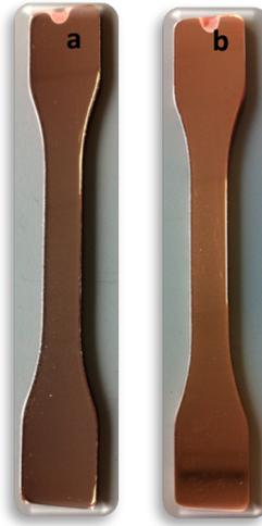
**Figure 4.5** Copper films deposited at  $0.4i_{p,\text{lim}}$  and (a)  $\theta = 0.25$ ,  $t_p = 100$  ms; (b)  $\theta = 0.50$ ,  $t_p = 100$  ms.
