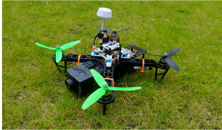
Figure 1.2: A typical racing drone – A 210mm racing drone fitted with standard equipment. Image Credit: Author.
