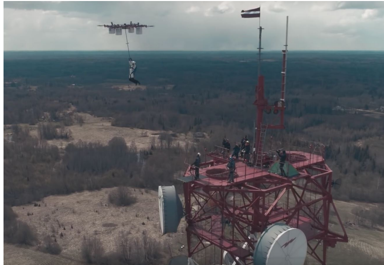
Figure 1.1: Skydiving from a multirotor – An example of a vehicle capable of lifting a human skydiver was successfully tested May 2017. Image Credit: Aeronex.
