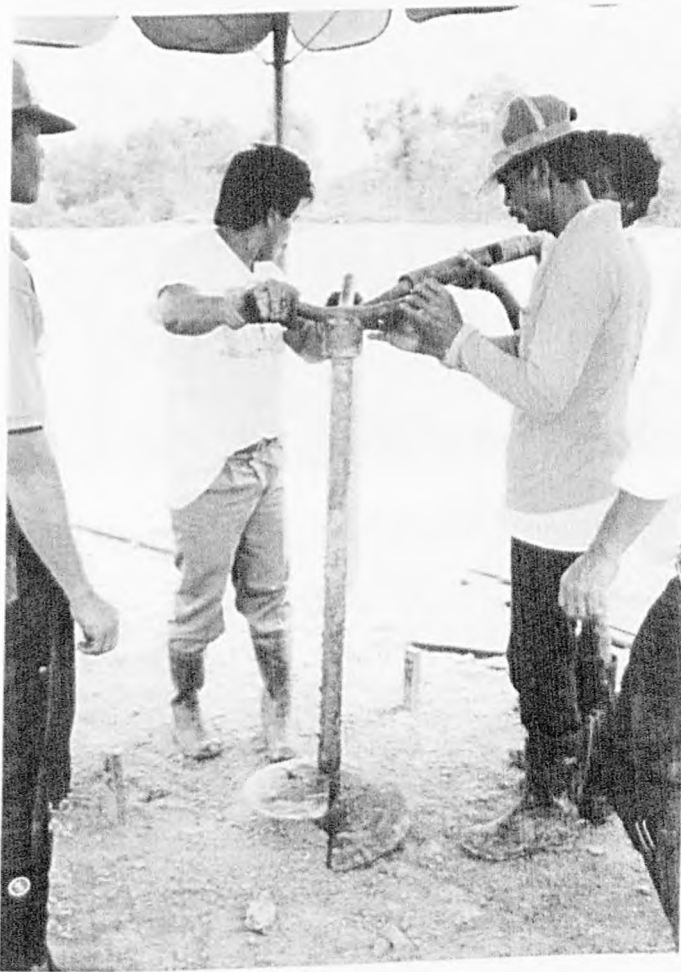
Plate 4.19 : Augering of Hole for Field Vane Testing
