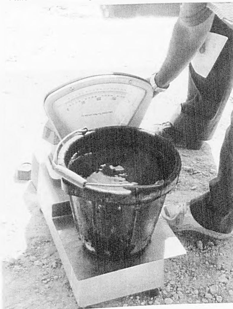
Plate 4.25: Water is Weighed Prior to Filling of Hole
