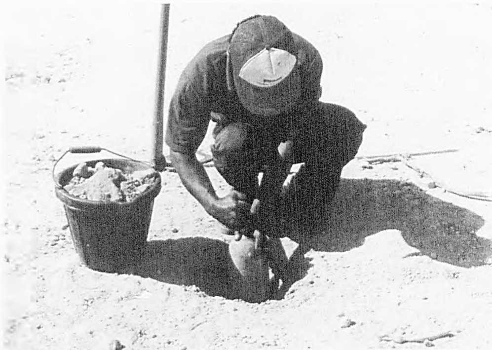
Plate 4.24: Hole Dug for Water Replacement Method
