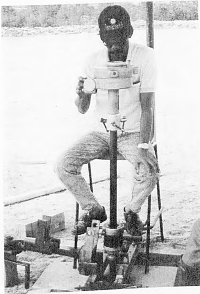
Plate 4.21 Shearing of the Soil During Field Vane Testing
