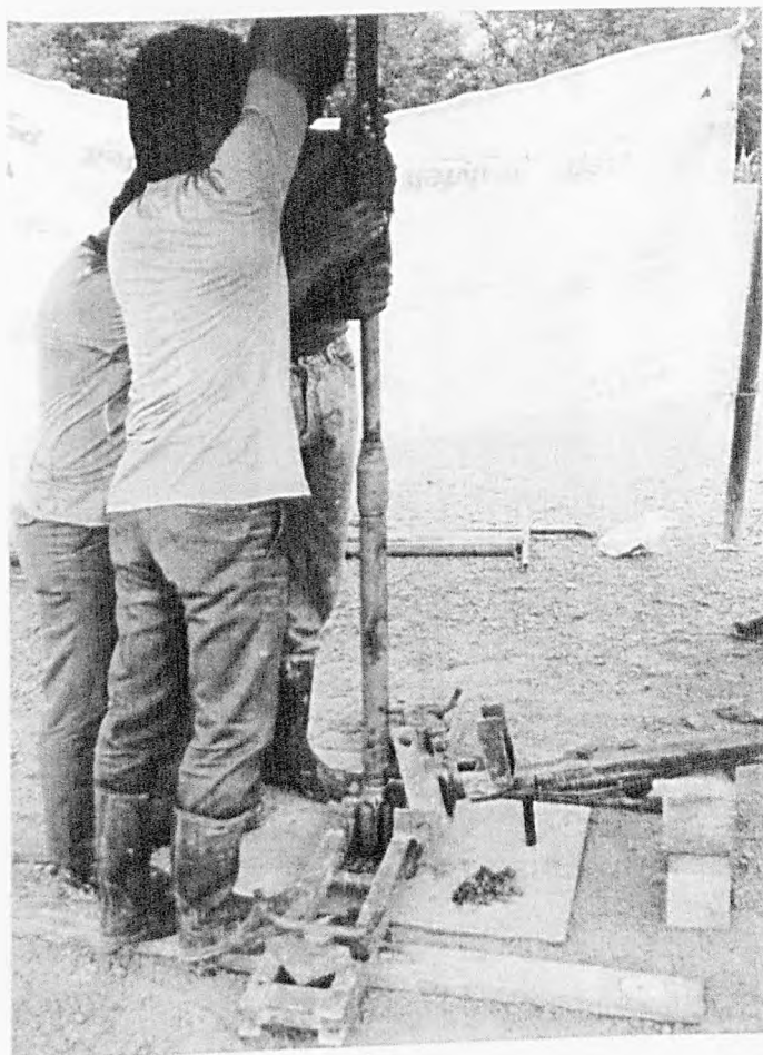
Plate 4.20 : Insertion of the Vane Tip for Field Vane Testing
