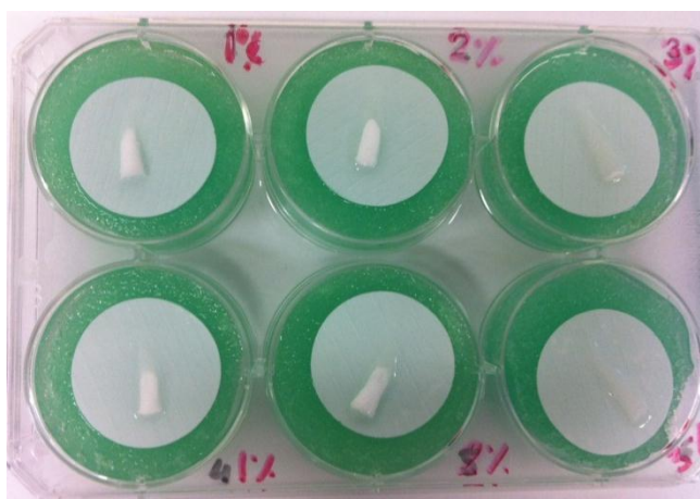
Figure 3.20. Photograph of a plate from the moisture uptake assay for inserts containing 1% (left), 2% (middle) and 3% CB[7] (right), taken after 10 min. The formulations containing 3% CB[7] appears to be gelling more quickly than those containing 1% or 2%.
