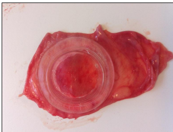
Figure 4.25. Photograph showing a donor chamber being fixed to the porcine nasal tissue with cyanoacrylate glue. Excess tissue was then cut away.
