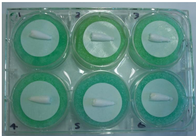
Figure 3.7. The set up for a moisture uptake experiment using sponges saturated in the absorption media and the inserts placed on a nylon membrane.
