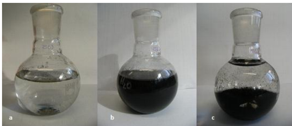
Figure 2.12. Images of ~ 20 mg f -CNT in a 100 mL round-bottom flask after: (a) no sonication, (b) direct contact sonication for 20 min, and (c) being further diluted with water and left to stand for a number of days. Note that in image (b) the f -CNTs were swollen, not fully dispersed, after 20 min, apparent from the opaqueness of the solution. After being left to stand for a number of days the f -CNTs have settled but remain swollen c.f. the starting image.
