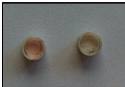
Figure 4.16. Photographs of the samples after TGA analysis. The formulation containing K6 (left) had turned pink. The insert containing K6@CB[6] remained white (right).
