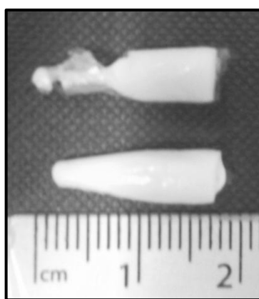
Figure 5.6. Image of lyophilised nasal inserts containing cisplatin, lyophilised using Method 2 (top) and Method 3 (bottom). The top insert shows shrivelled morphology, indicating meltback.
